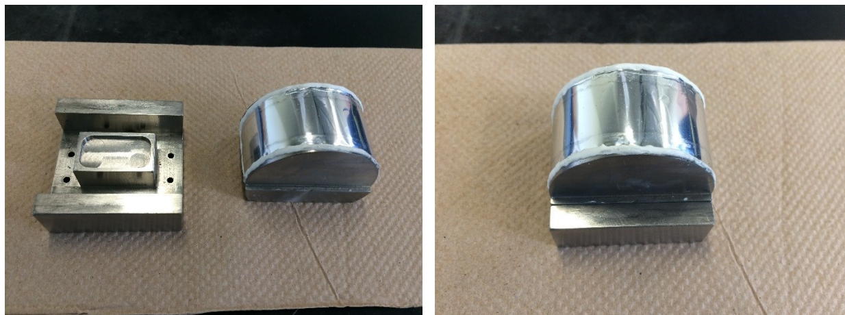
Figure 3.3 Air sensitive XRD holder before (left) and after (after) assembly
