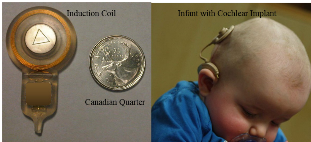
Figure 1: Implanted portion of a cochlear implant powered through magnetic induction (left) and photograph of a pediatric cochlear implant patient (right)
