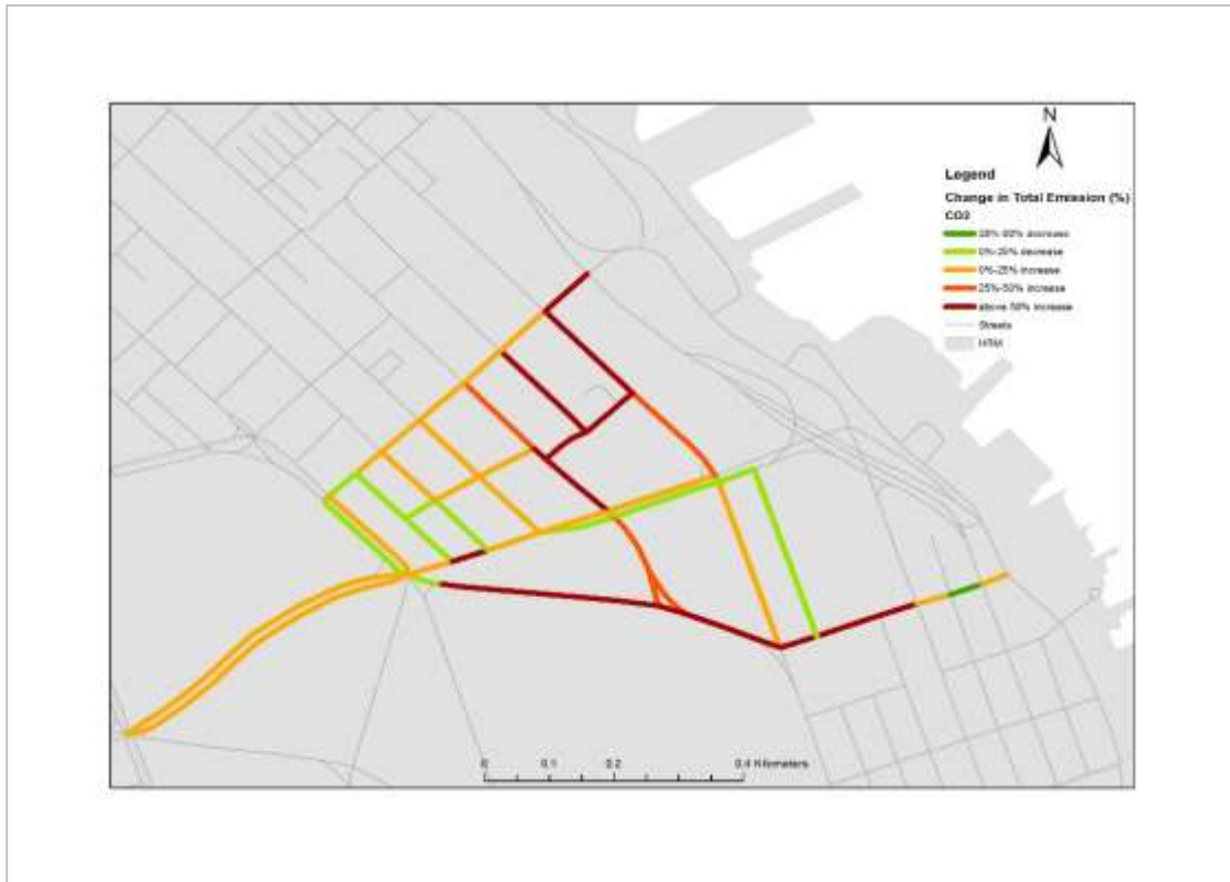
Figure D1 Changes in Total Emissions (g) of GHG in AM Peak Period
