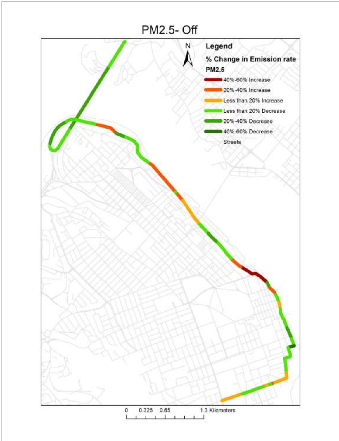
Figure A8 Relative Difference in PM 2.5 Emission Rates from Link Average Emission Rate in Off Peak
