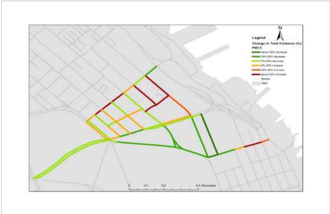
Figure D12 Changes in Total Emissions (g) of PM 2.5 in Off Peak Period
