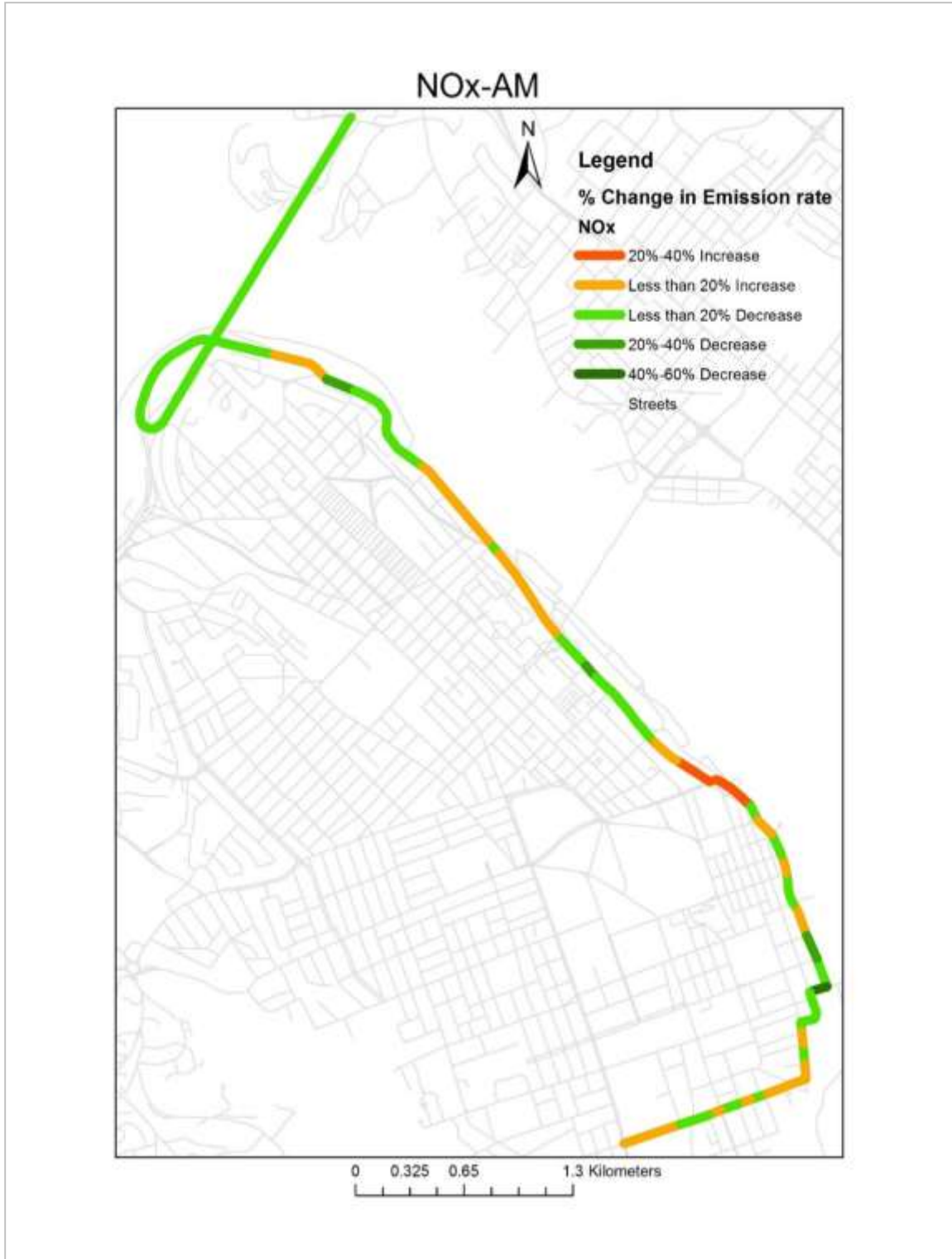
Figure 2-7 Relative Difference in NOx Emission Rates from Link Average Emission Rate in AM Peak
