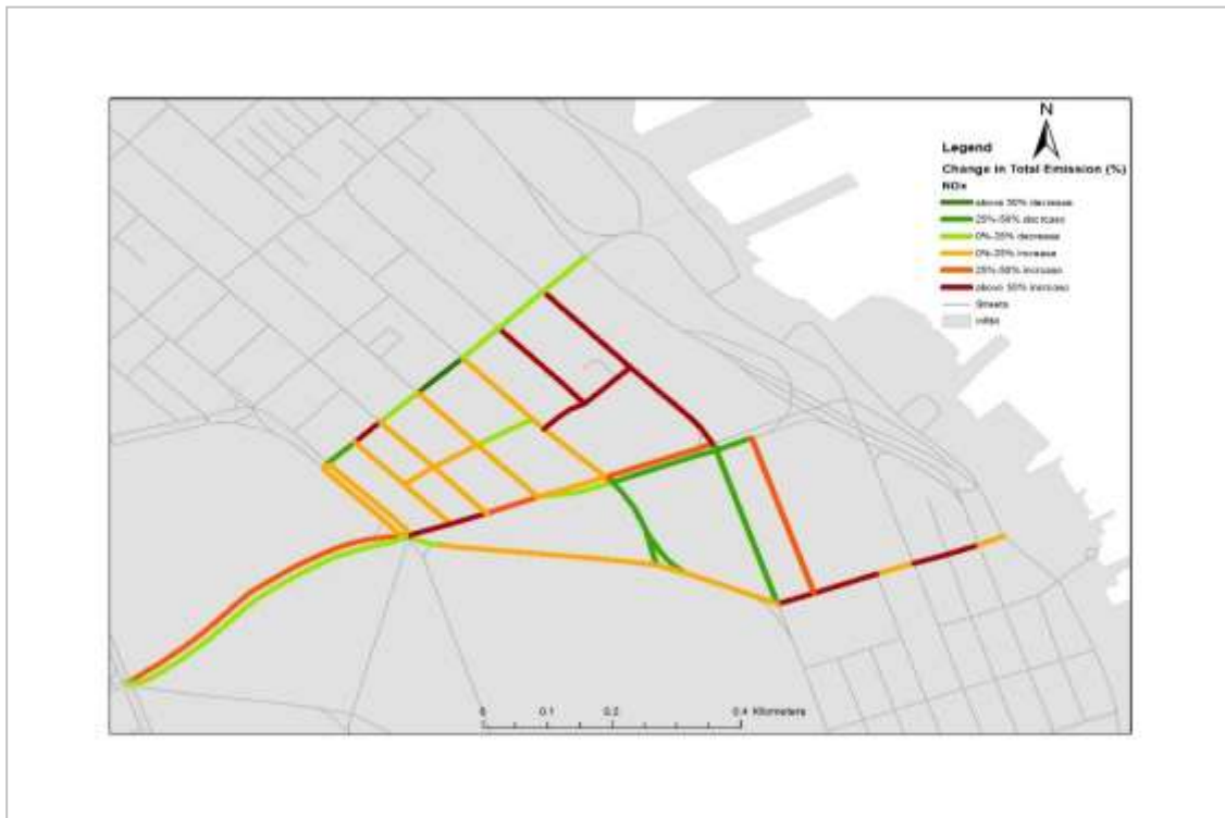
Figure D15 Changes in Total Emissions (g) of NOx in PM Peak Period
