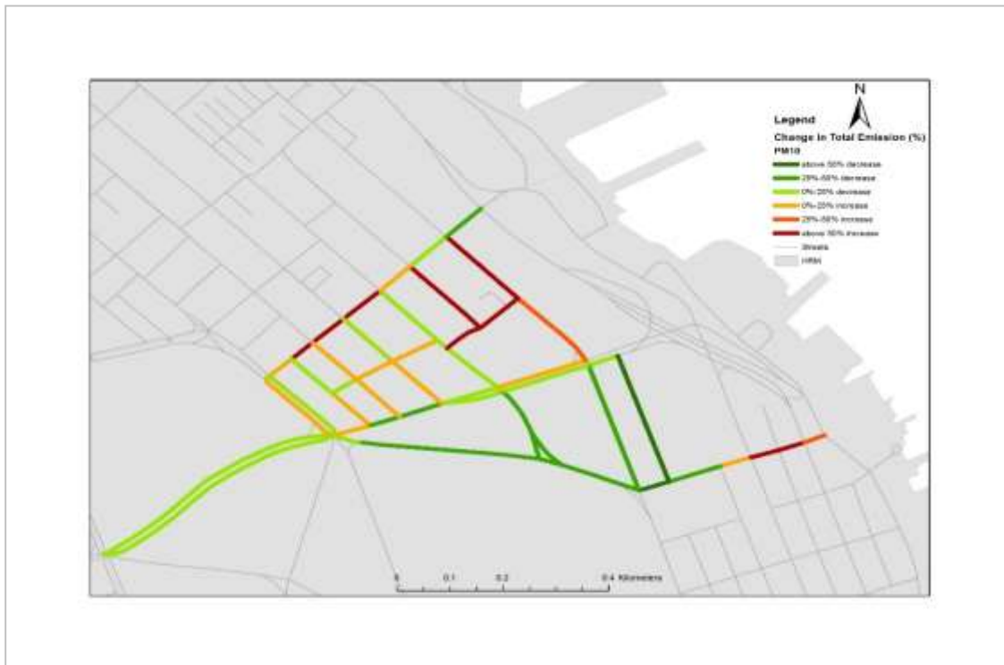
Figure D11 Changes in Total Emissions (g) of PM 10 in Off Peak Period
