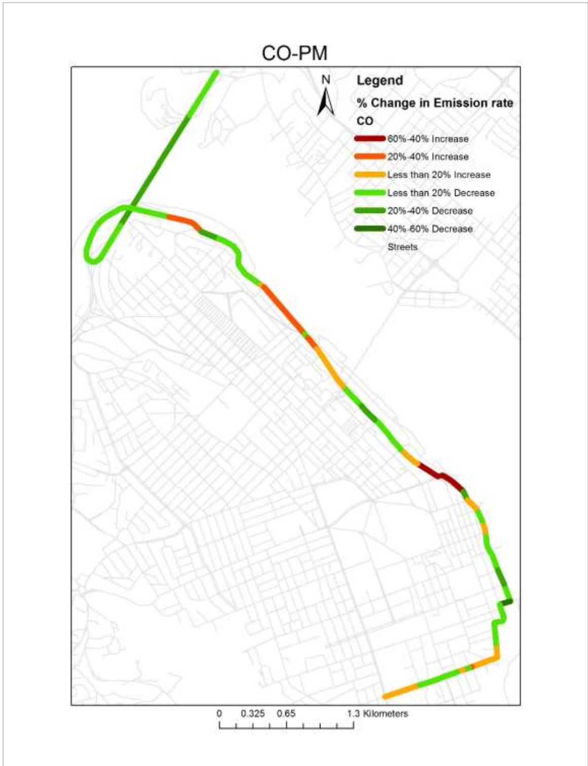
Figure A9 Relative Difference in CO Emission Rates from Link Average Emission Rate in PM Peak
