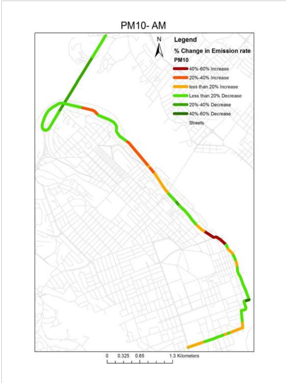
Figure 2-8 Relative Difference in PM 10 Emission Rates from Link Average Emission Rate in AM Peak
