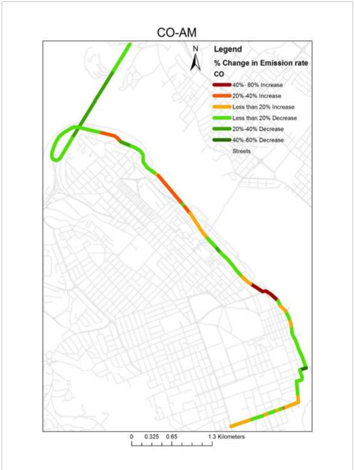
Figure 2-6 Relative Difference in CO Emission Rates from Link Average Emission Rate in AM Peak
