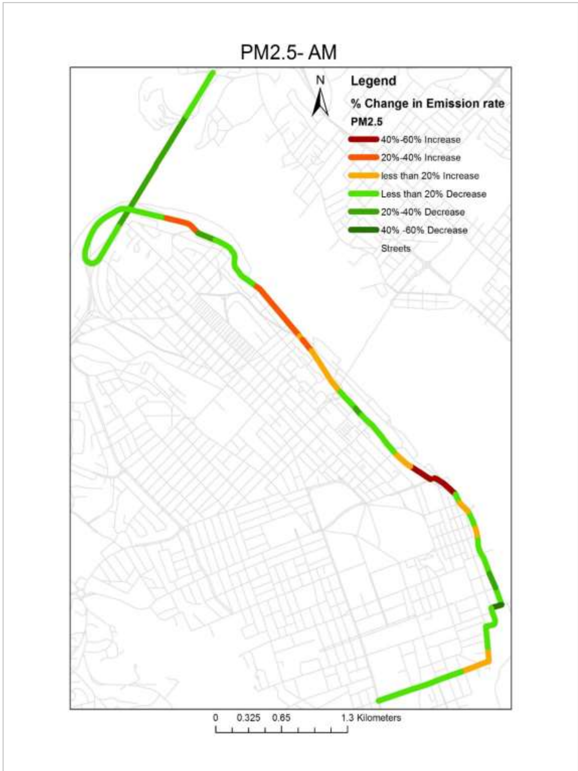
Figure 2-9 Relative Difference in PM2.5 Emission Rates from Link Average Emission Rate in AM Peak
