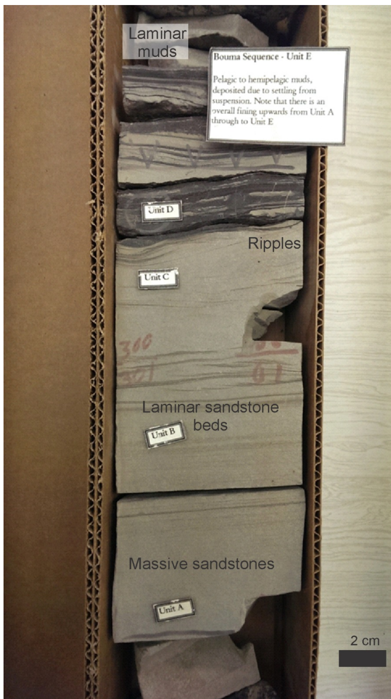
Figure 2.4: A typical Bouma fining-upward sequence. Photo taken at the Bureau of Economic Geology (BEG) Core Center, Houston, Texas.
