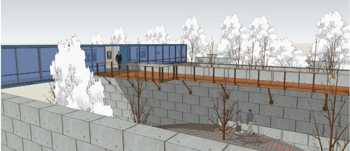
Two 40' containers placed as a temporary gallery across 3 sections of wall with walking paths below.
