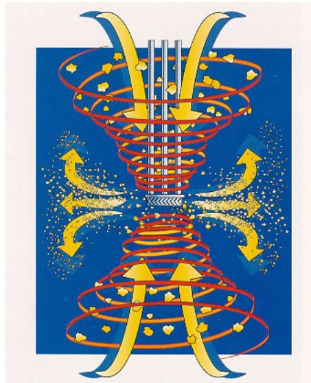
Figure 2-4. The vortex created by rotating blades [4]
