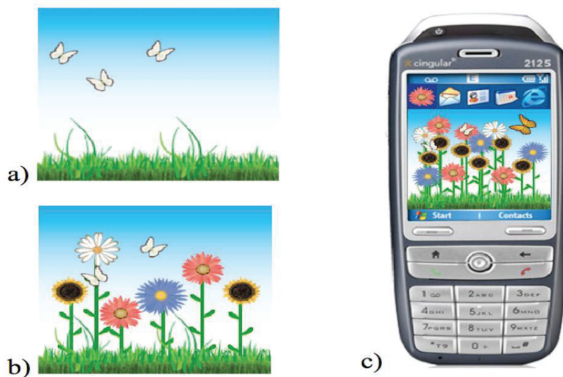
Figure 2.2: UbiFit Garden's glanceable display [38]: a) at the beginning of the week-small butterflies indicate recent goal attainments; the absence of flower means no activity this week; b) a garden with workout variety; c) the display on a mobile phone- the large butterflies indicates this week's goal was met.
