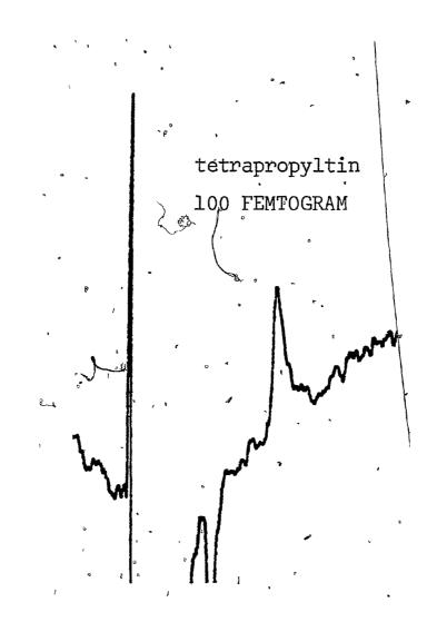
halides and acids by conversion to their corresponding hydrides, in combination with the very sensitive photometric tin detector and gas chromatography, was attempted at Dalhousie. A novel approach was taken, using a gas mixture of 0.5% silane in ultra-high purity nitrogen, as reagent.
