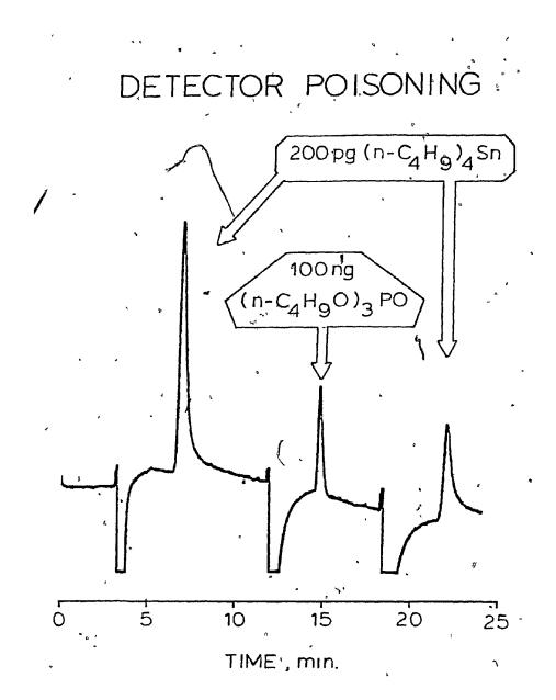
caused by the prior injection of 100 nanograms of tributylphosphate. Fortunately, good detector response for tin can be restored by the introduction of fluorocompounds into the operational FPD.
