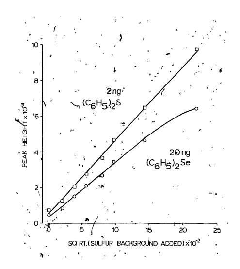
a linear relationship is obtained for the sulfur analyte:  $R_{\rm S} = k_{\rm S}^2 S_{\rm A}^2 + 2k_{\rm S} S_{\rm A} \sqrt{B}$  (13) and  $k_{\rm S}$  can be determined from the slope  $2k_{\rm S}S_{\rm A}$ . The values found for  $k_{\rm S}$  by the two methods, as expected, were
