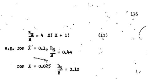
Using equation 11, a simple calculation shows that in order to stay within a 10% deviation from linearity, the analyte peak must not be larger than about half (44%) of the sulfur-induced background. If the peak measures only 10% of the background, the deviation from linearity will be less than 2.5%, i.e. insignificant for any practical purposes. Similar considerations could be applied to selenium or tellurium analytes on selenium or tellurium backgrounds.
