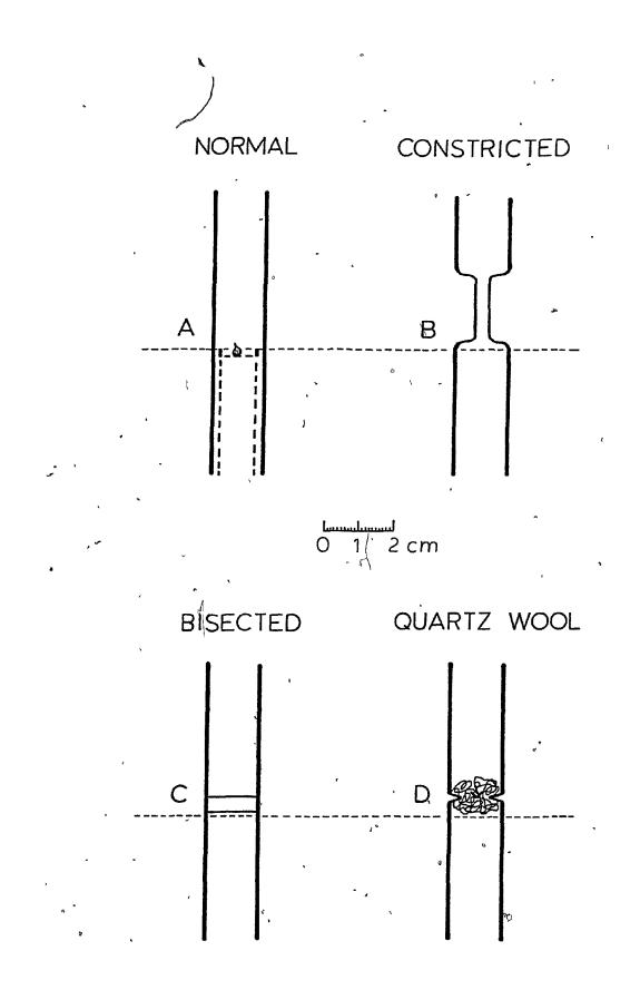
normal cylindrical enclosure to a smaller diameter in the region of view of the PM tube. The effect of the diameter of the collapsed region on tin response was determined by making several tubes with constrictions of varying diameters. Enclosure C was developed to test the hypothesis that tin emission is a surface luminescence phenomenon. A normal flame enclosure was bisected with a much smaller diameter guartz tube (3.5 mm OD) so
