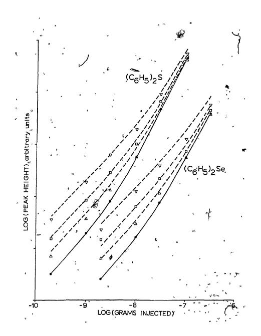
the calibration curves of selenium on sulfur was similar to that of sulfur on sulfur, suggesting a similar mathematical treatment. In a purely formal analogy, a binomial expression could be written,
