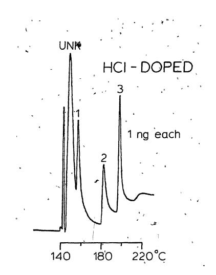
each type of compound and this was accomplished by using a low carrier gas flow rate (e.g. 10 ml/min) and longer columns. For very heavy compounds such as triphenŷltin chloride and dioctyltin dichloride, which elute very late off most columns, the effect of column temperature on reaction is not important. Shorter, faster columns are preferred to allow these compounds to elute at reasonable temperatures.
