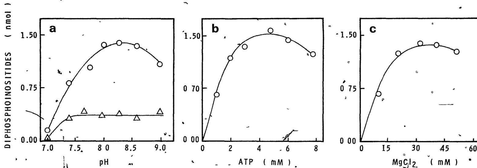
Fig. 20: Effects of pH(a), ATP(b) and MgCl<sub>2</sub>(c) on PIK Activity. Standard assay conditions. using 2% Cutscum with 3 min incubation time. o, 8-day chick brain (0.95 mg protein); Δ, 11 day chick sciatic nerve (0.61 mg protein).
