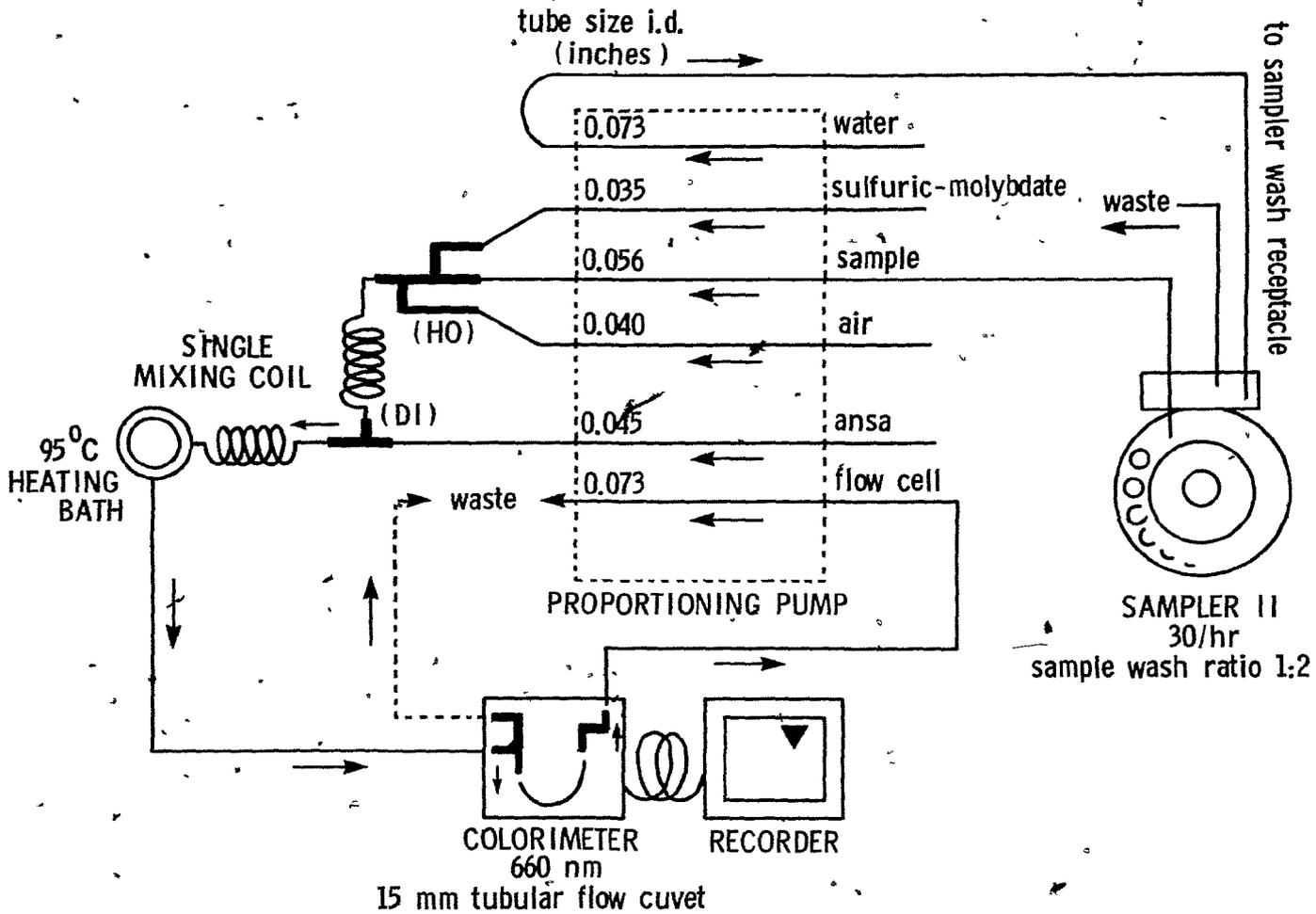
(e).. Continuous Flow Manifold for Determination of Total Phosphate.
