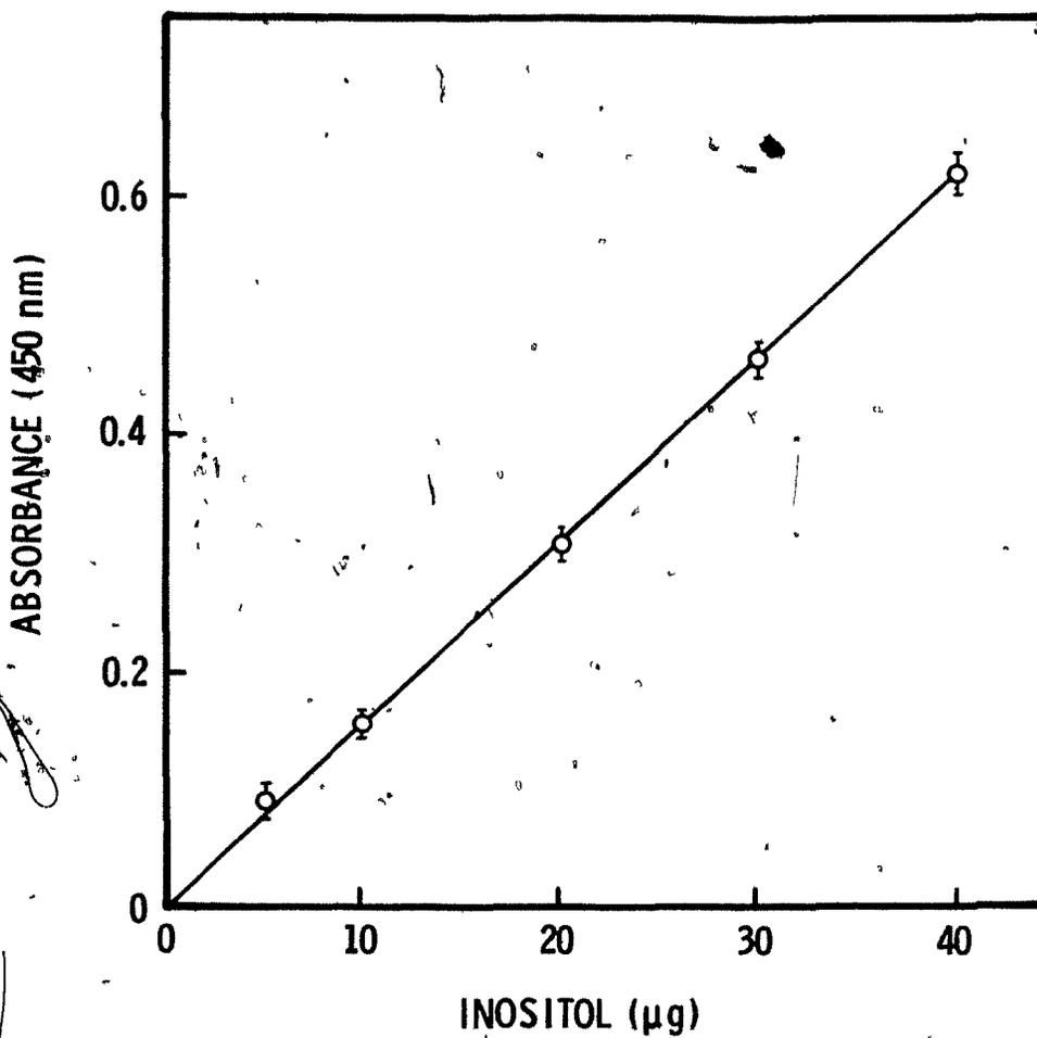
Fig. 12: Inositol Standard Curve by the Chemical Method. Values represent the mean  $\pm$  S.D. for 10 determinations.
