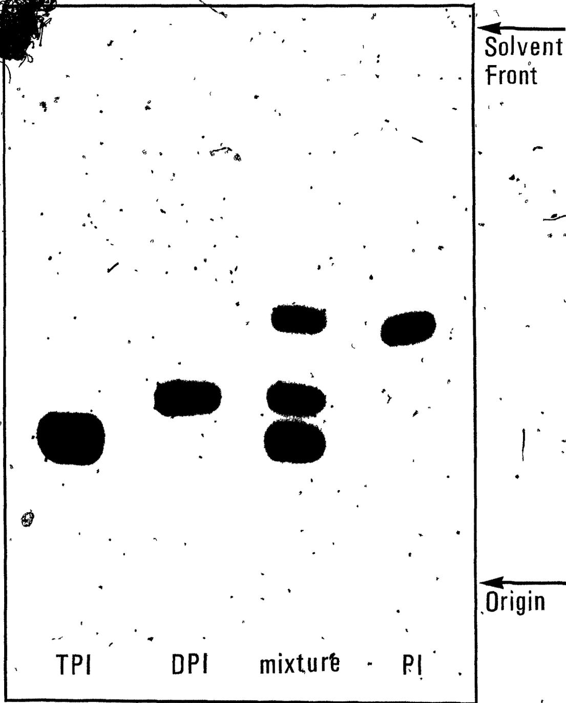
Fig. 7: Thin-Layer Chromatography of Pure DPI and TPI Prepared by DEAE-Cellulose Column Chromatography. Lipids (in  $\mu\text{g P}$ : TPI, 8; DPI, 5; PI, 5 and mixture of three lipids in the same amounts) were chromatographed on Silica Gel H plate impregnated with potassium oxalate (see Methods 4b & c).
