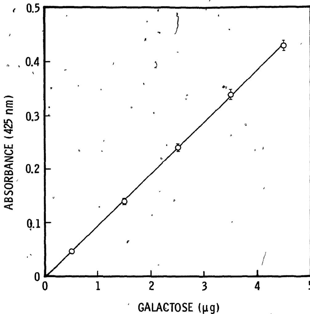
Fig. 9: Galactose Standard Curve as Determined by the Orcinol-H<sub>2</sub>SO<sub>4</sub> Method. Values represent the mean  $\pm$  S.D. (where S.D. is of sufficient magnitude to plot) for 7 determinations.
