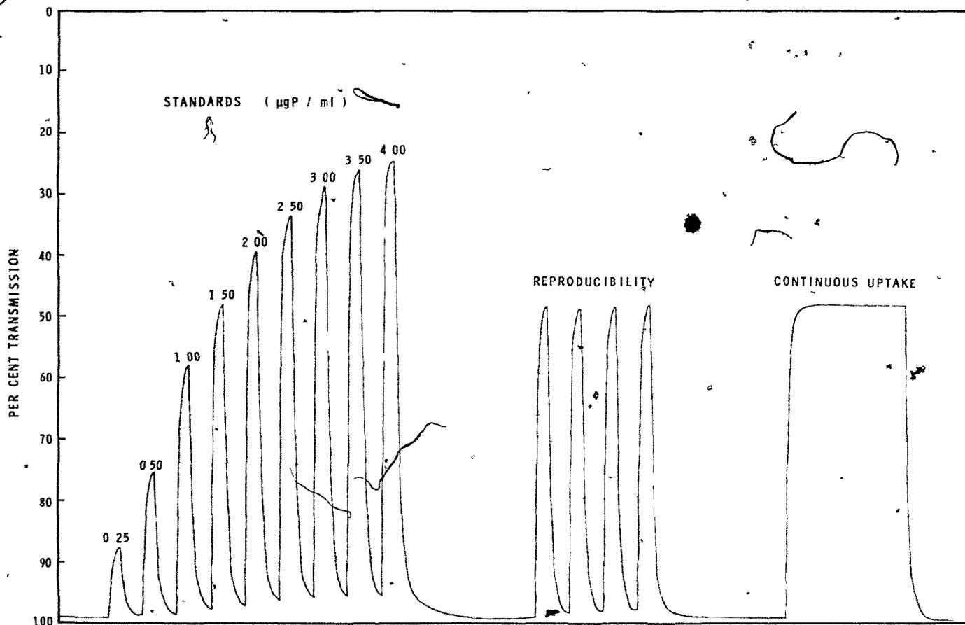
(b) Actual Tracings of Pi Determination Showing Standards, Reproducibility, Peak Separation and Continuous Uptake.
