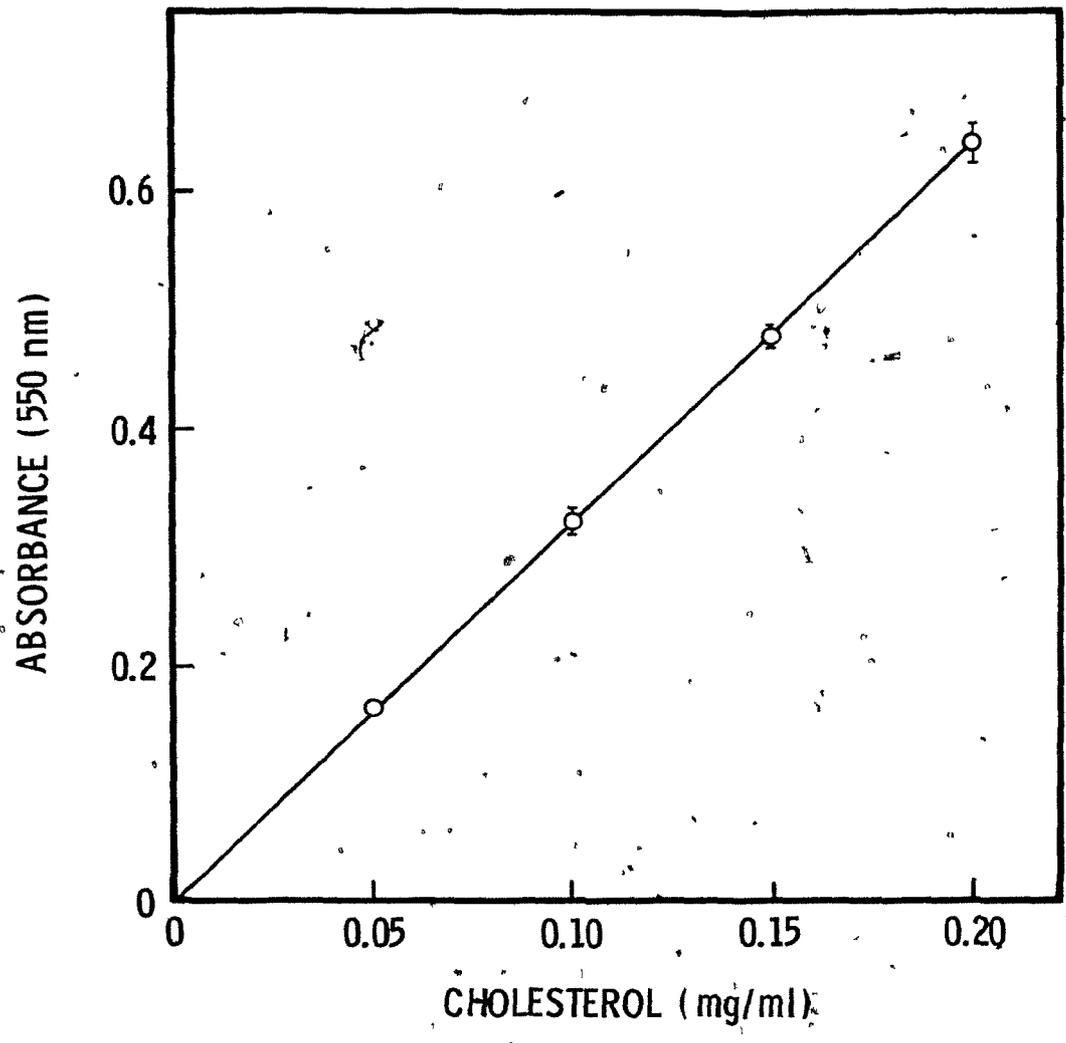
Fig. 8: Cholesterol Standard Curve as Determined with the Technicon Autoanalyzer. Values represent the mean  $\pm$  S.D. (where S.D. is of sufficient magnitude to plot) for 7 determinations.
