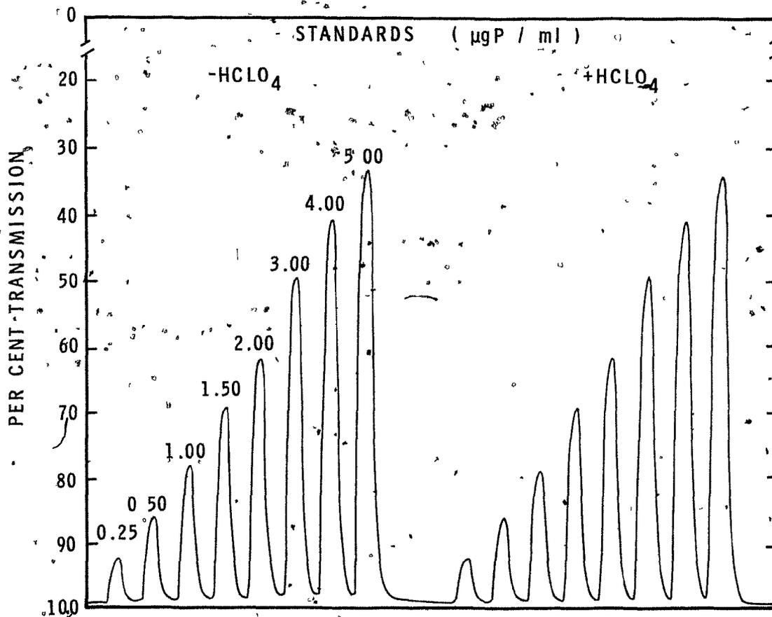
(g) Effect of Acid on Profile of Total Phosphate Estimation (see text for detail).
