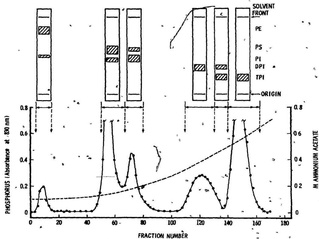
Fig. 6: DEAE-Cellulose Column Chromatography of Bovine Brain "Enriched Sodium Polyphosphoinositide" Fraction. Fractions were examined by t.l.c. using Silica Gel HR plates containing oxalate, developed in C-A-M-AA-W (40:15:13:10:7, by vol.). (●), Phosphorus measured; (---), gradient of ammonium acetate (calculated).
