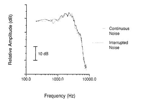
Figure 5: Root-mean-square amplitude spectra of the continuous and interrupted broadband noise, as a function of frequency (Hz), delivered to a 2 cm<sup>3</sup> HA-2 coupler from an insert earphone.
