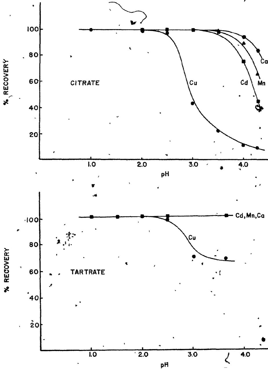
Fig.4-10: Pre-column uptake as a function of pH.
