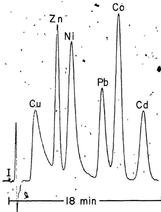
Fig. 3-2: Isocratic A-9/tartrate separation.
