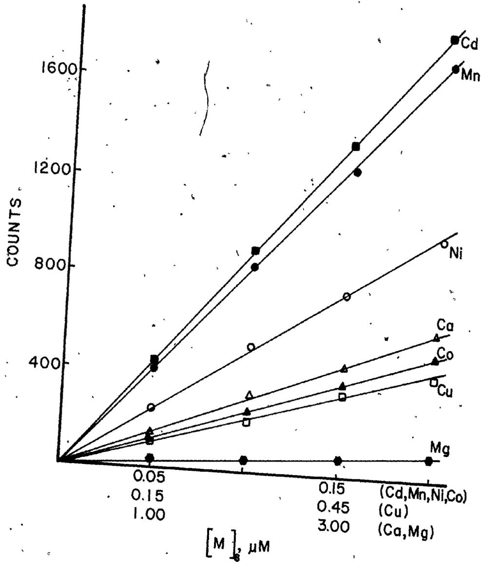
Fig. 4-8: 20x pre-concentration into 0.01 M EDTA.
