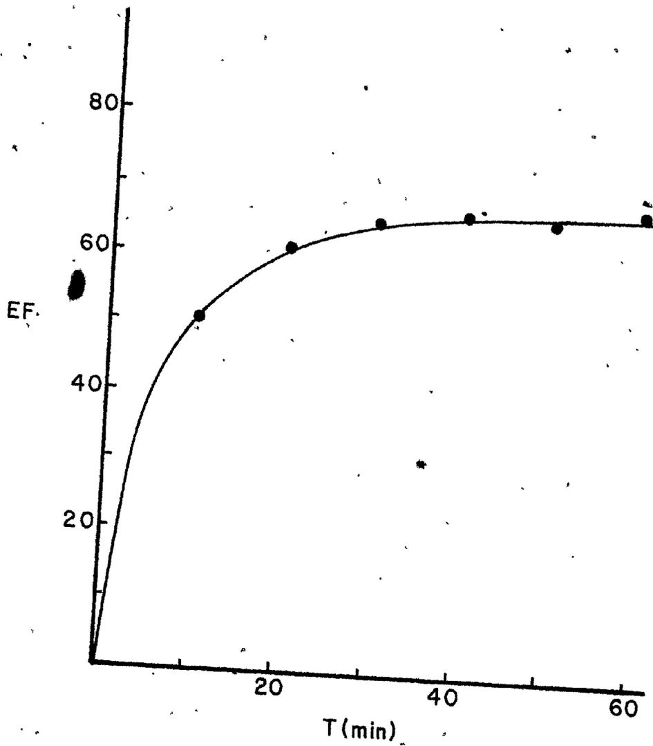
Fig.4-5: A 200/2 preconcentration of Zn into 0.20M tartrate (pH 3.74).
