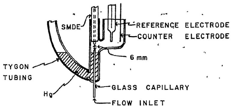
Fig. 2-5a: HMDE detector
