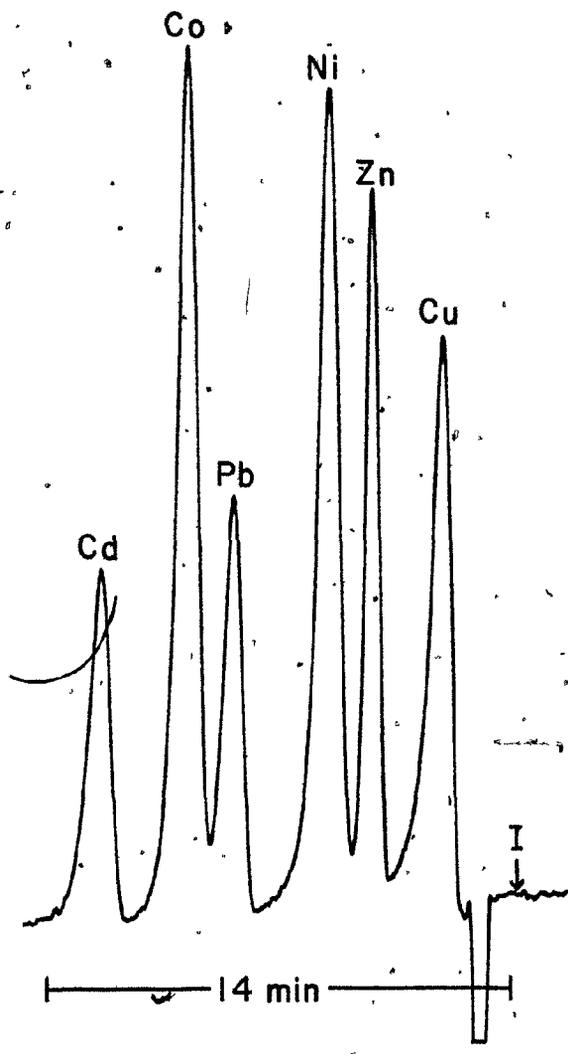
Fig. 3-3: Isocratic A-8/tartrate separation.
