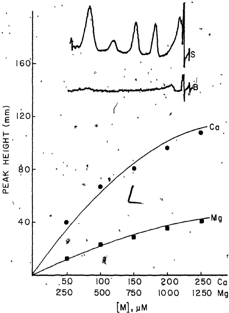
Fig. 3-8: Calibration curves with A-9/citrate.
