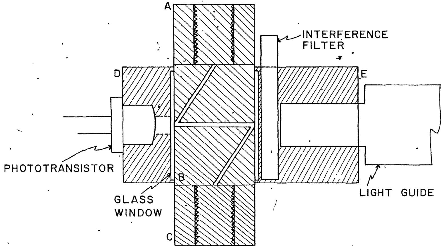
Fig. 2-3: Top view of flow cell
