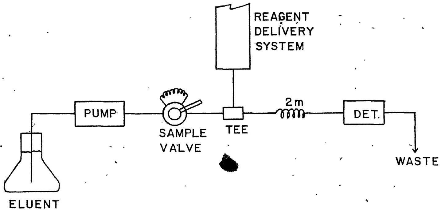
Fig.2-1: Flow injection system for comparison of detectors .
