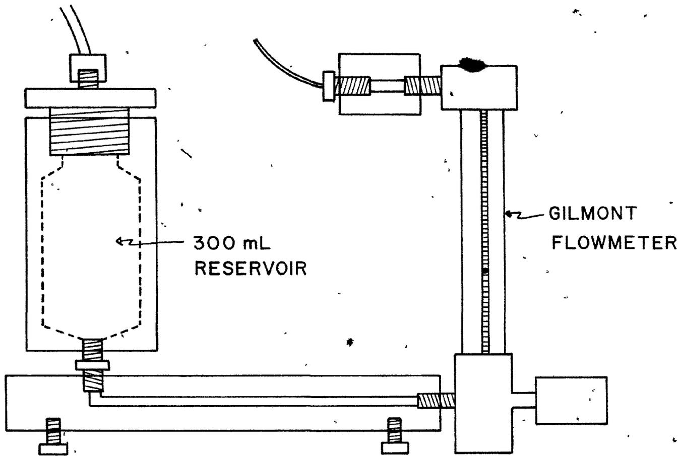
Fig. 2-2: Pressurized delivery system .
