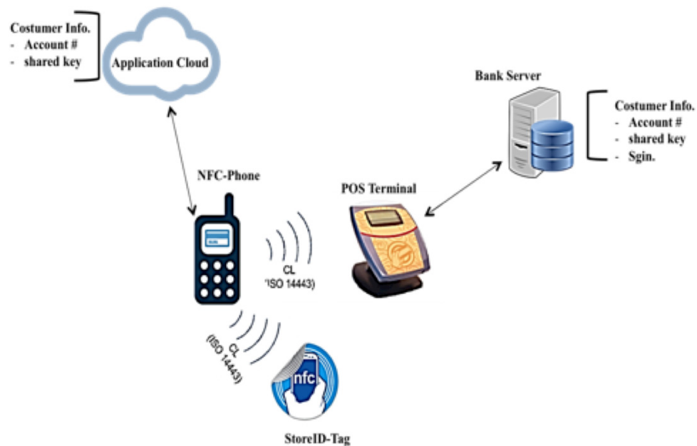
Figure 4.1 the architecture of the proposed system.
