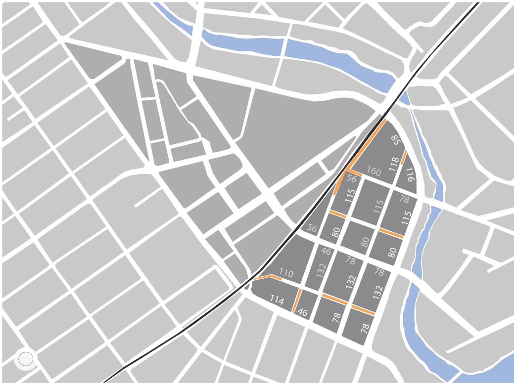
New Block Breaks New streets added to reduce the size of large blocks and eliminate dead-end conditions; data from Bartholomew, municipal CAD files
