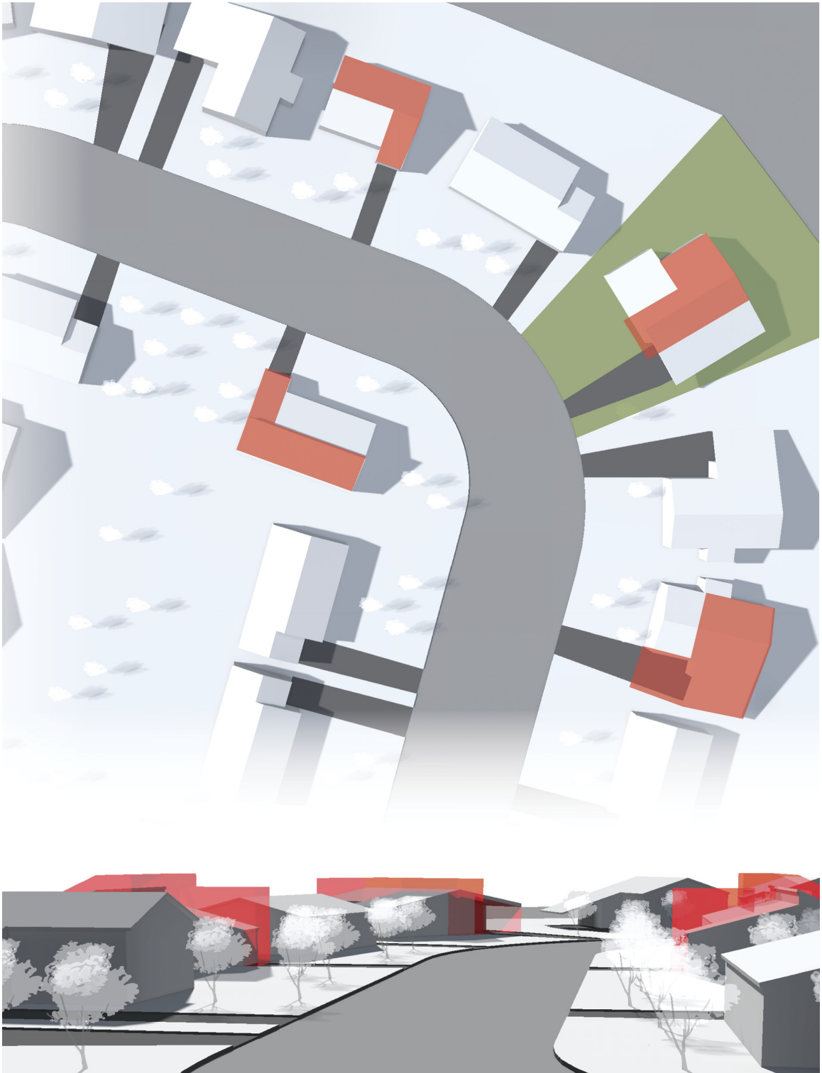
Fig. 50 A smart growth strategy which addresses scale within the neighbourhood while also providing additional amenity space within each unit.
