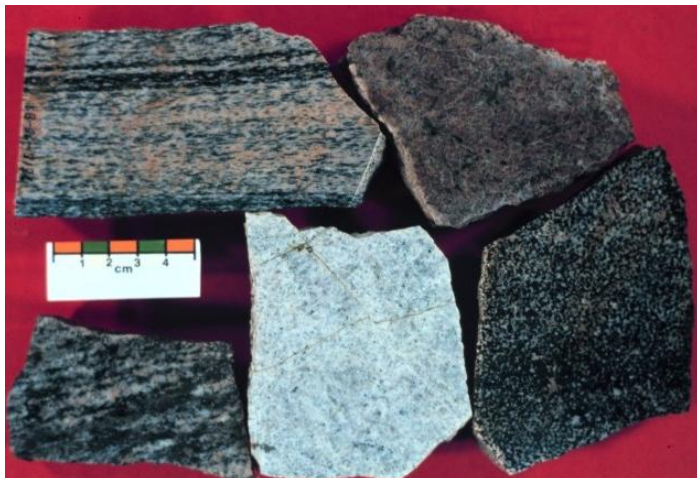
Figure 4-11. A selection of cut slabs from the Blair River inlier. Upper and lower left: orthogneiss; upper right, syenite; lower middle, anorthosite; lower right, ferrogabbro. Mafic minerals are darker grey/black.
