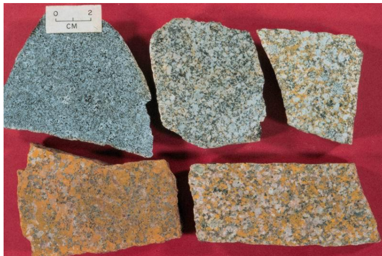
Figure 4-6. A selection of cut slabs from the ca. 620 Ma plutons in Mira terrane, ranging in composition from diorite (upper left) to syenogranite (lower left). Slabs have been etched and stained to emphasize K-feldspar (yellow), plagioclase (white), and quartz (grey). Mafic minerals are dark grey/black.
