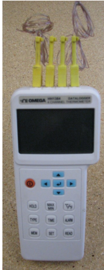
Figure 3.4 Thermocouples and Portable Data Logger
