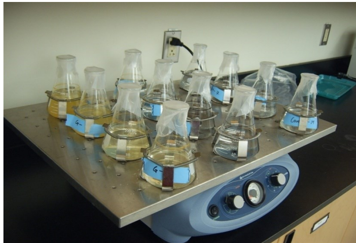
Figure 3.15. DOM adsorption study using goethite and magnetite in synthetic water samples at lab temperature and 150 rpm.
