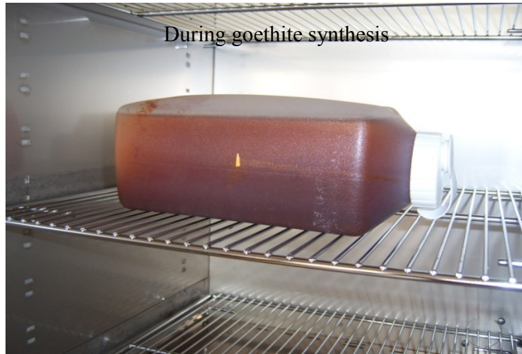
Figure 3.2. Preparation of goethite ( \alpha -FeOOH) in an oven placed at 70 °C for 60 h.
