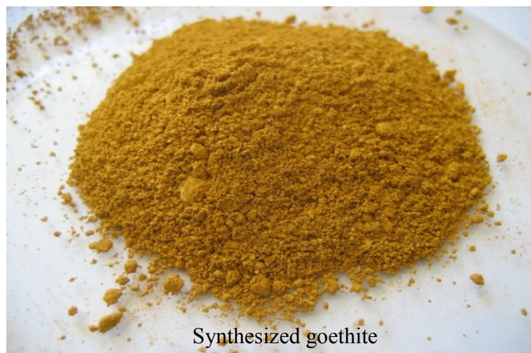
Figure 3.3. Synthesized goethite sample ( \alpha -FeOOH) after air dried.
