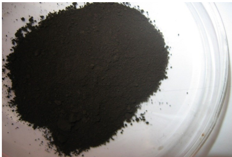
Figure 3.8. Synthesized magnetite sample ( \text{Fe}_2\text{O}_3 ).
