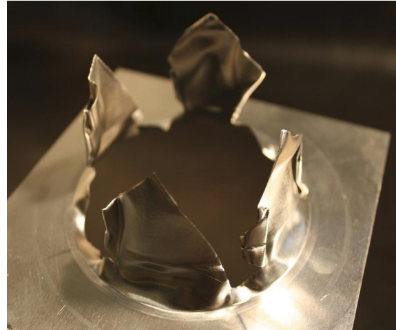
Fig. 12. Burst aluminum diaphragm.
