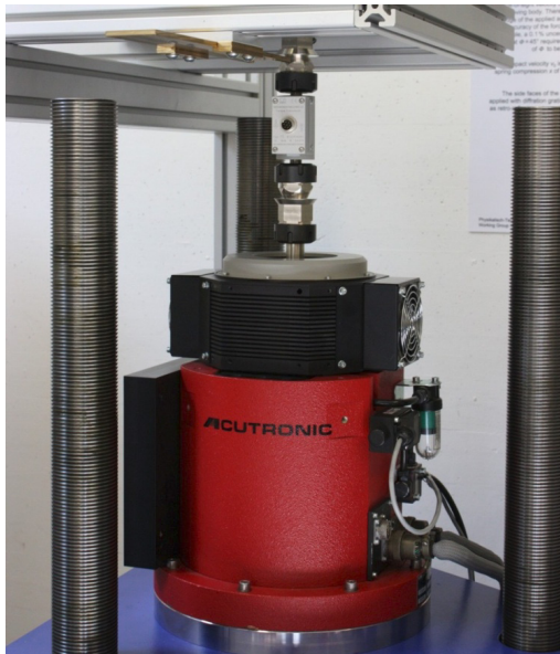
Fig. 13. Dynamic torque measuring device at PTB with the new rotational exciter.
