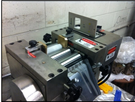
Fig. 3.4 The three-roll mill equipment used in the calendering process.
