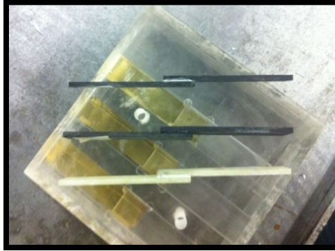
Fig. 3.7 Typical graphite/epoxy and glass/epoxy single-lap joint specimens.
