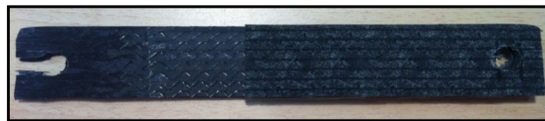
Fig. 3.10 Tearing-off problems in SLJs that were without quasi-isotropic tabs as a result of being subjected to tensile impact loading.
