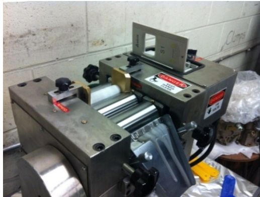
Fig. 4.4 The three-roll mill equipment used in the calendering process (Torrey Hills Technologies LLC, San Diego, CA).
