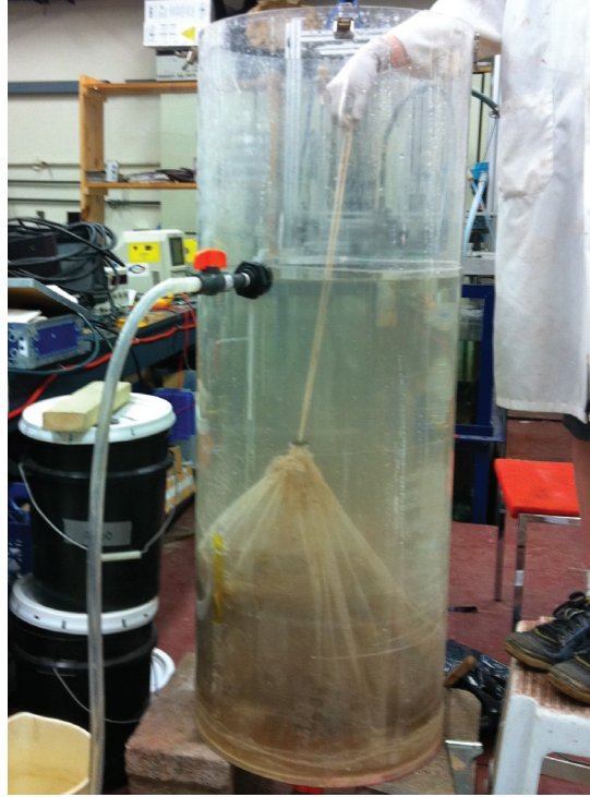
Figure 3.3: The water displacement apparatus with a sample block that has sunk in the fresh water. The block is contained within a mesh bag.
