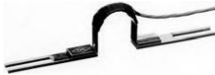
Figure 4.4 - PI crack gauges (Tokyo Sokki Kenkyujo Co. Ltd., 2011)
