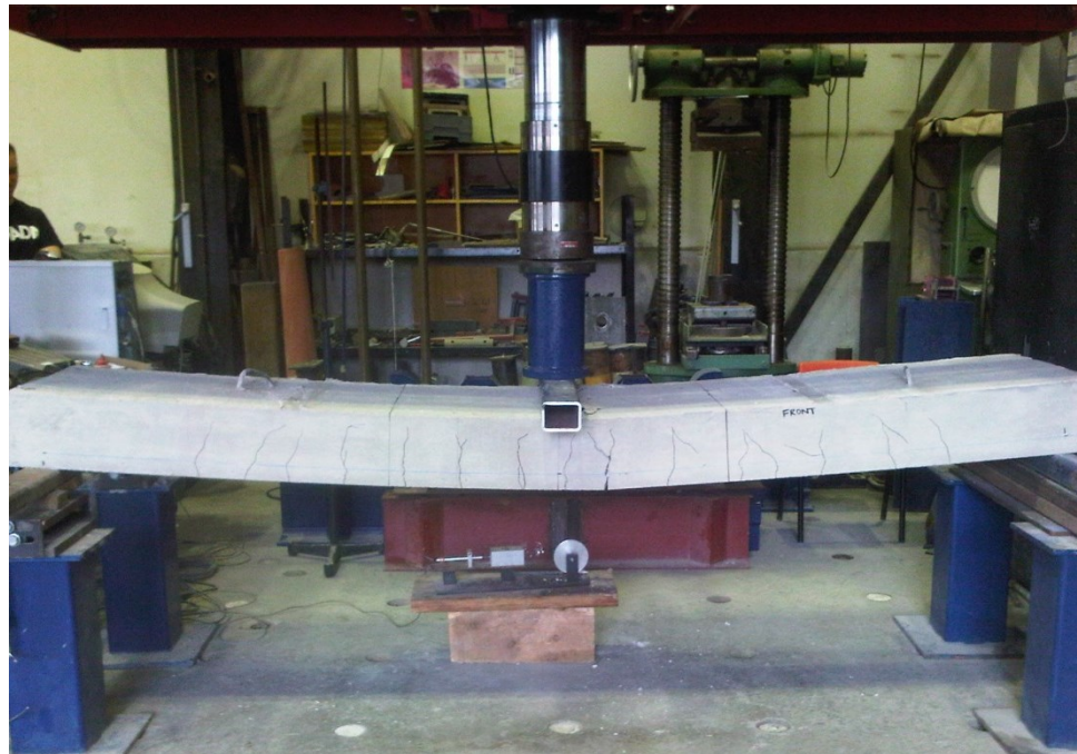
Figure 4.5 - Failure Arrangement for Slabs S1 – S8
