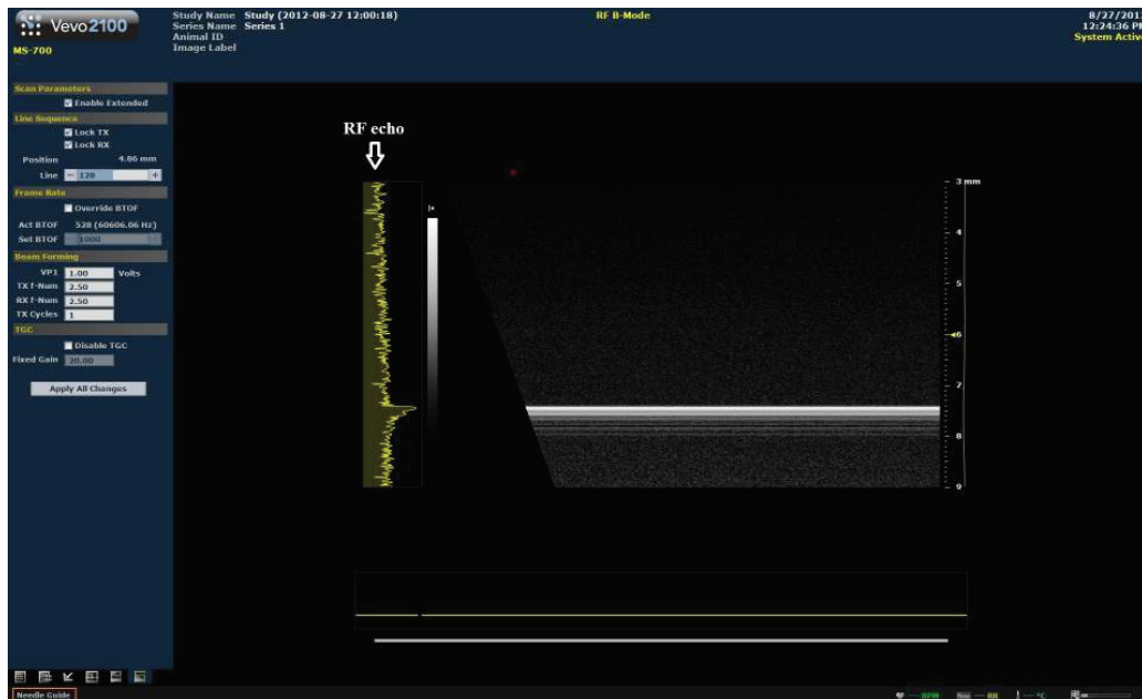
Figure 4.9: A screen shot of the extended engineering mode on the Vevo 2100. The central 64-elements of the array are collecting one focused RF line steered to 20 degrees. The RF echo is marked with the arrow and this line is repeated producing the B-mode image displayed.
