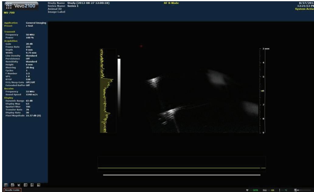
Figure 4.8: B-mode image of two 30\mu\text{m} wire targets when the beam is steered to 20 degrees, captured with Vevo 2100. Since the pitch of this array is greater than .5\lambda , grating lobes are present in the field of view when the beam is steered.
