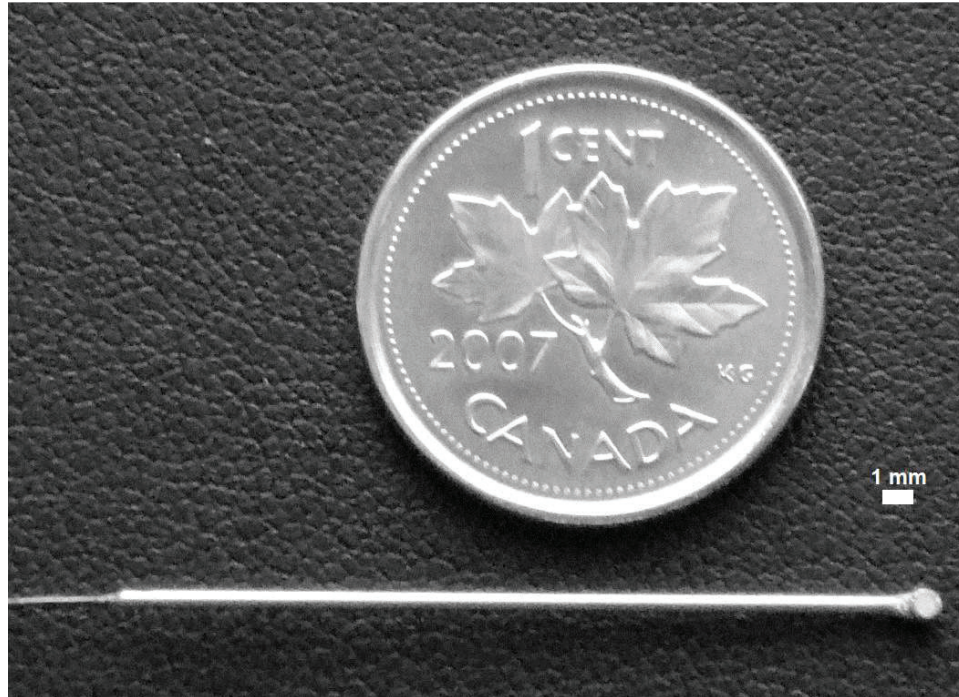
Figure 5.3: Photograph of needle Doppler probe (Torbatian et al. (2012b), with permission of the Elsevier).
