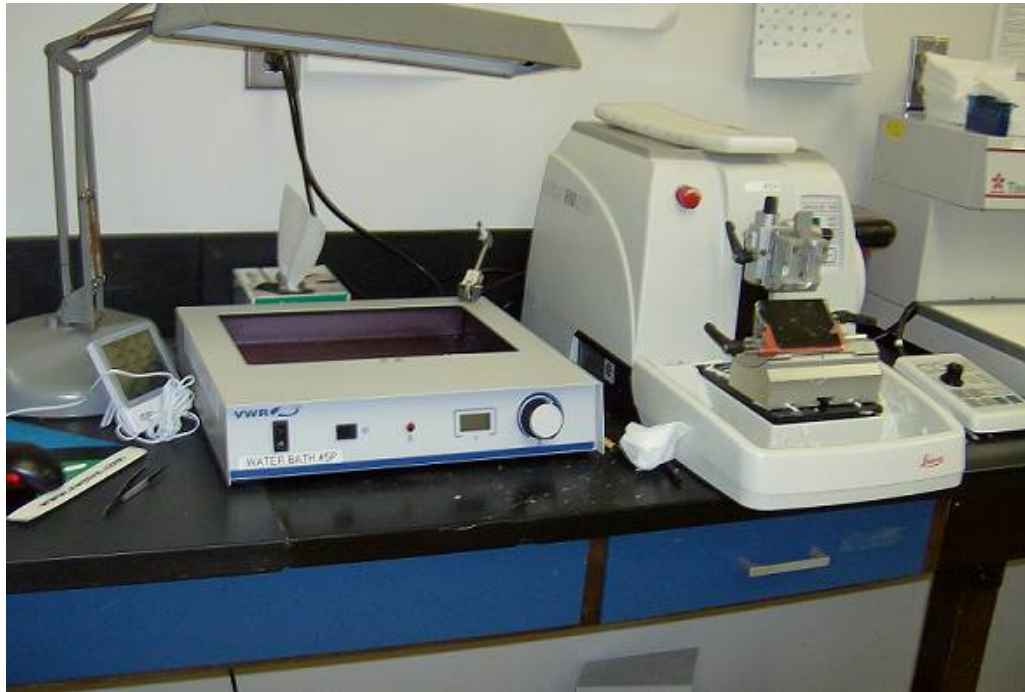
Figure 4.5: Microtome (right) and water bath (left) used to cut and place intestinal sections on slides.
