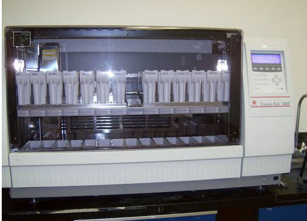
Figure 4.6: Tissue-Tek ® DRS ™ used for haematoxylin and eosin staining intestinal slides.
