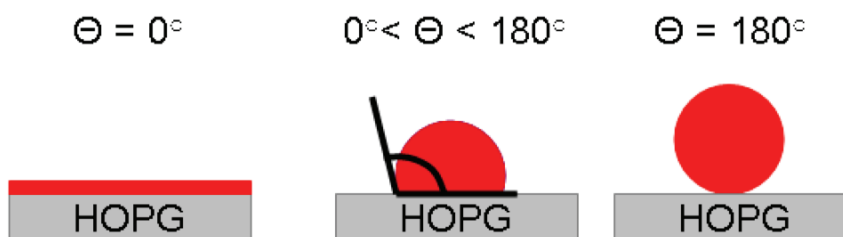
Figure 2.12: Schematic illustrations of contact angle at a solid-liquid interface. The images from left to right depict a solution that fully wets a solid, partially wets the solid and does not wet the solid. Image reproduced from Ref. [40]
