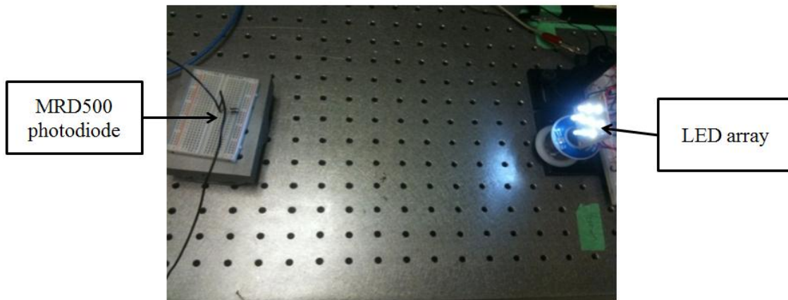
Figure 5.11: Testing the receiver performance for 50cm distance.
