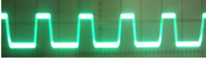
Figure 4.15: Output waveform from MAX3222 from Tout pin15.
