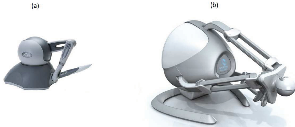
Figure 5.1: (a) Phantom Omni haptic device [62] and (b) Novint Falcon haptic device [61]
