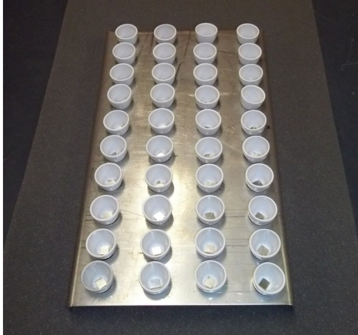
Figure 20 – Test setup with samples in glazed alumina crucibles prior to oxidation.
