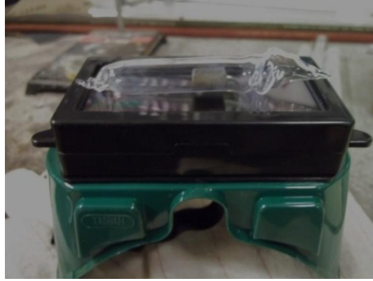
Figure 19 - Thermomechanically deformed 1 cm sample that has been prepared for ageing.
