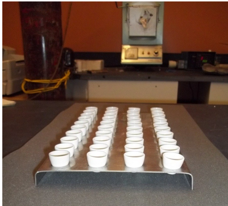
Figure 21 - Test setup crucibles in stainless steel tray prior to oxidation.
