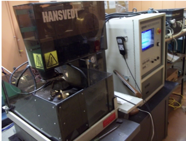
Figure 16 - Image of the traveling wire EDM used in the present research.
