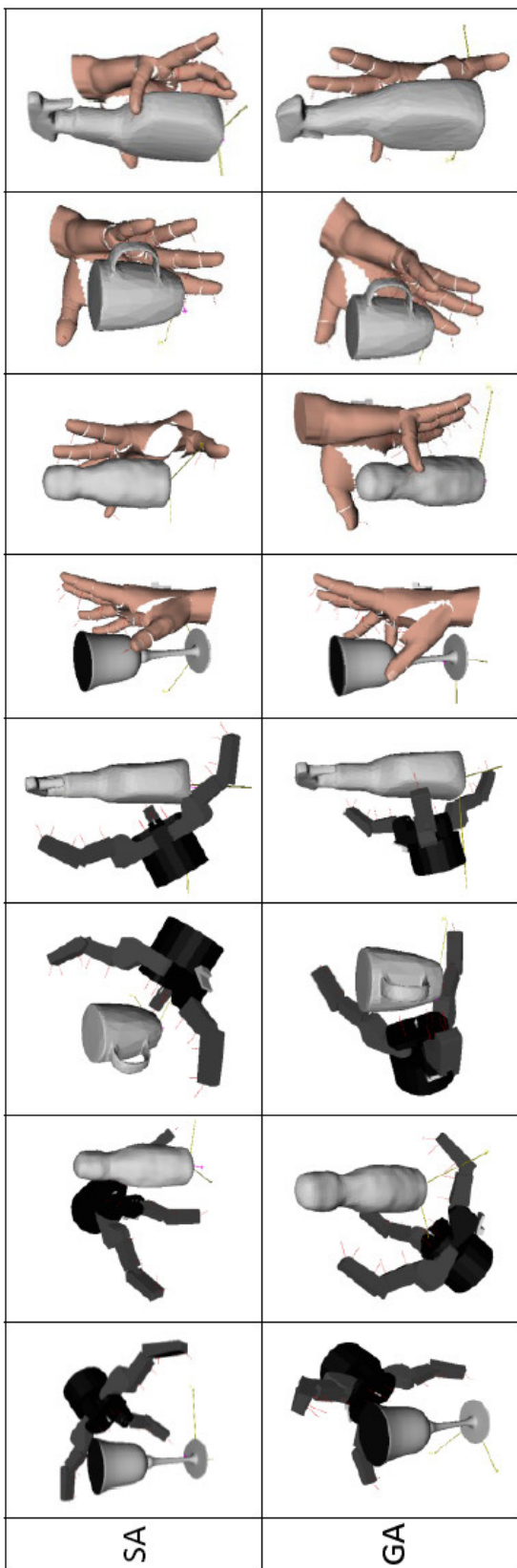
Figure 4.16: Best pre-grasps found by GA and SA planners with Q_{final} as the quality measure
