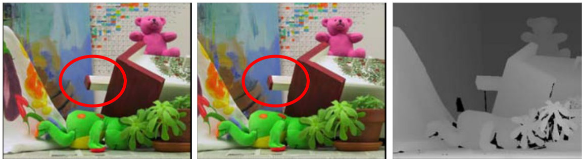
(a) Image from the left sensor (b) Image from the right sensor (c) Derived depth image
