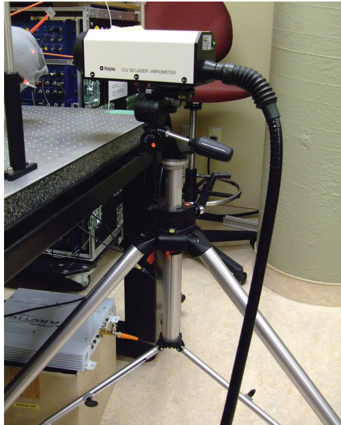
Figure 2.5: Polytec's 3D single point laser Doppler vibrometer (LDV) mounted on a tripod.
