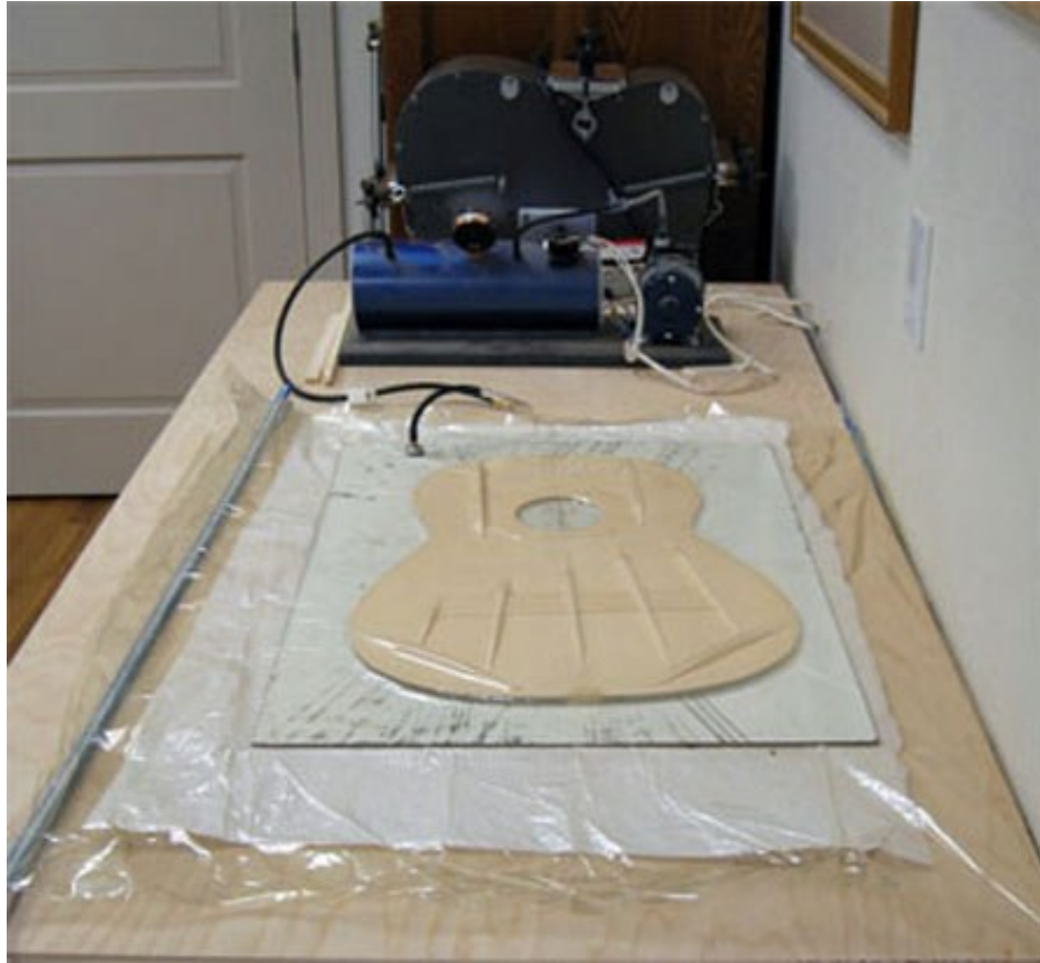
Figure 4 - Braces are glued to a guitar top inside a vacuum bag, (Scott, 2011)
