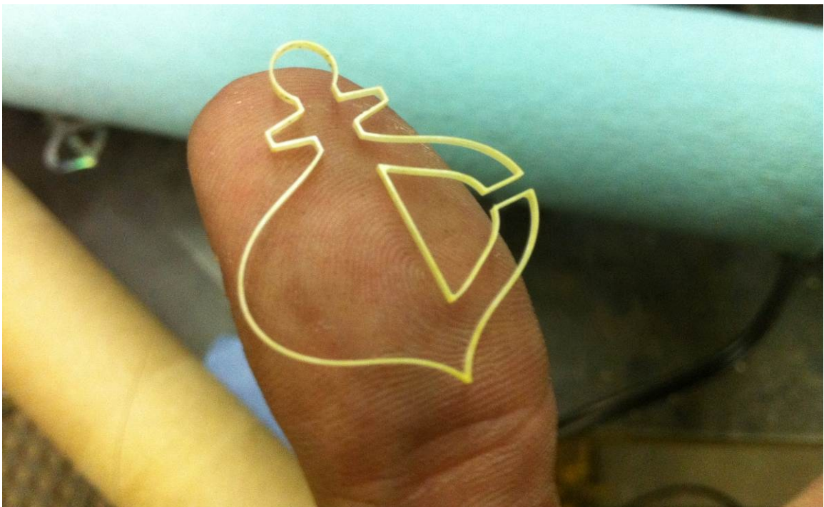
Figure 40 - Shell test piece. The piece fits inside a 28mm circle (standard Canadian Toonie), and line width is 0.014".
