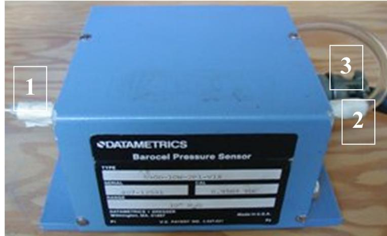
**Figure 2.5** Pressure transducer; 1- total pressure port, 2- static pressure port, 3- connected to the electronic manometer.
