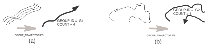
Figure 7.2: Illustration of two different version of operator GROUP_TRAJECTORIES (a) Group by Intersection, (b) Group by Overlap.
