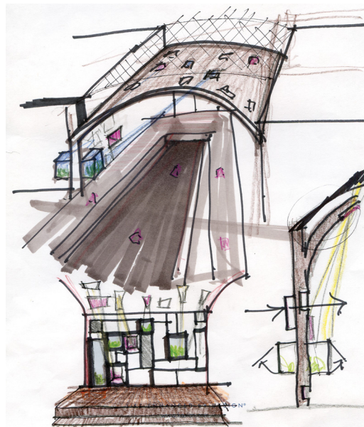
Sketches of the structure with light infiltration and double roof.
