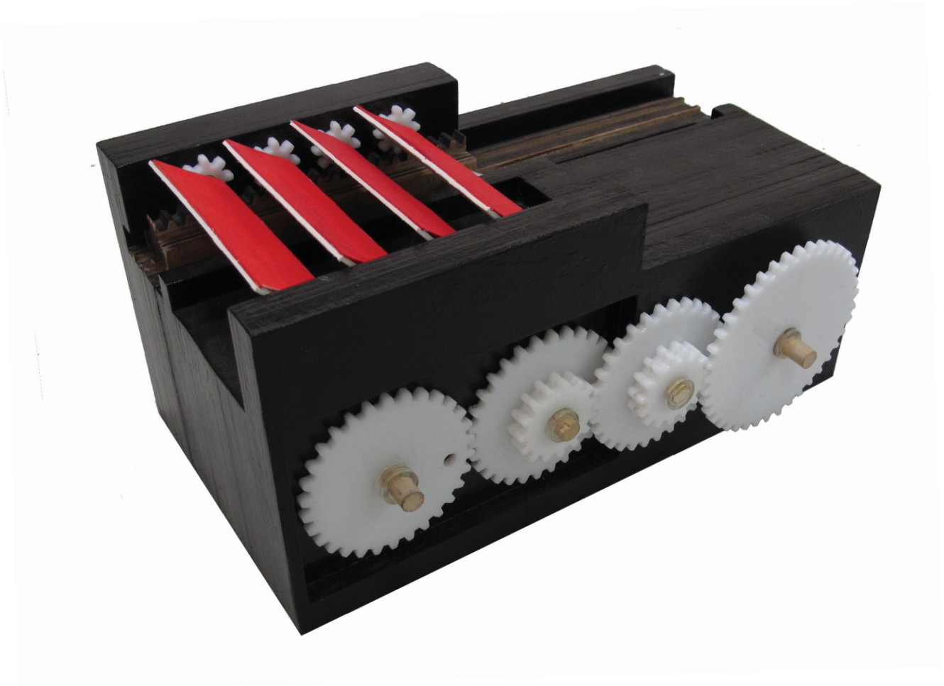
Study model of a gear mechanism designed to convert rotational motion to linear motion (like a crank and flywheel), eventually controlling the pitch of four louvers. Early idea for sun collection device.
