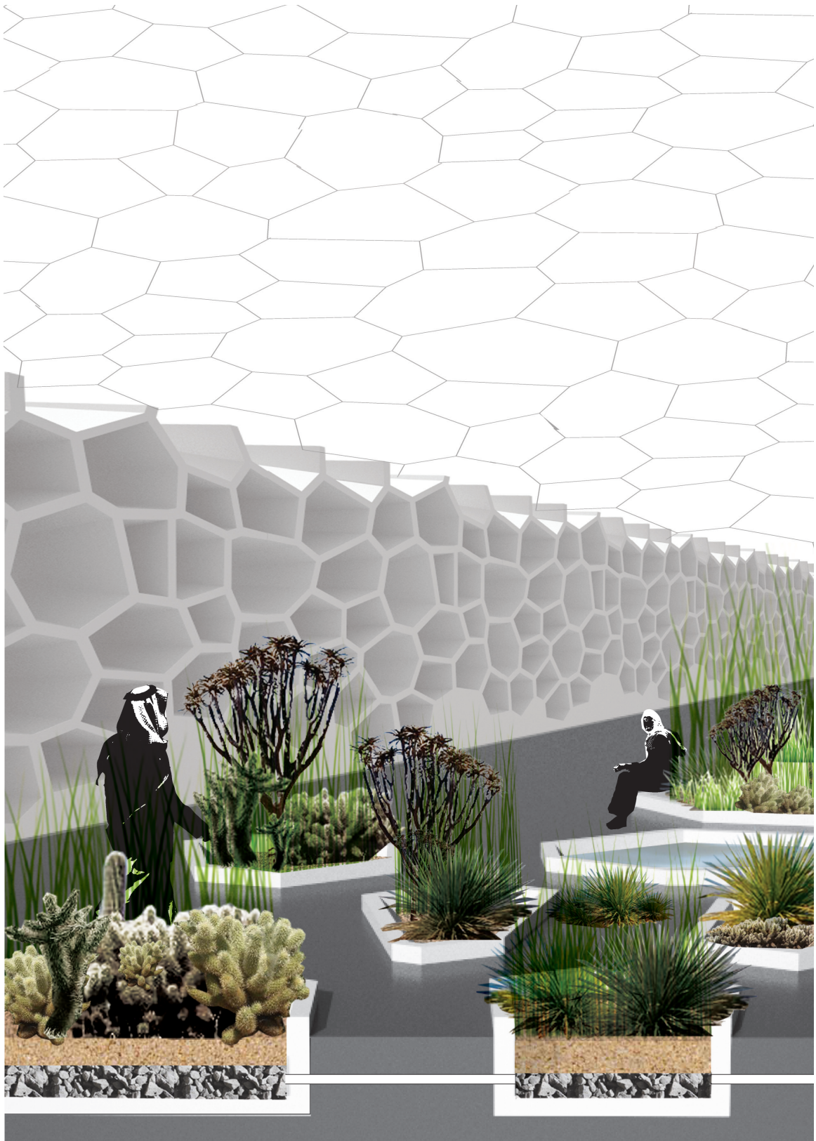
A view within the space, showing the garden plots, water pools and the connective piping which allows them to act as a grey-water treatment system.
