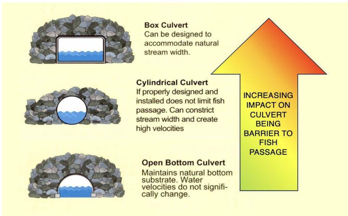
Figure 5.2 Culvert shape categories and impacts (DFO, 2015)
