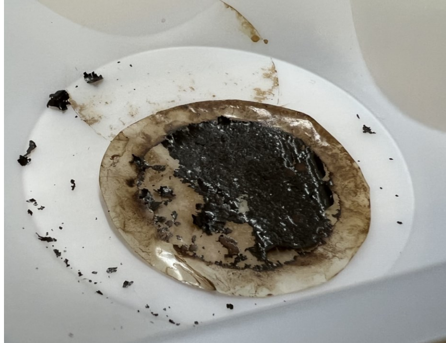
Figure 3.3. Example of particles over 1 \mu\text{m} filtered from solution dried on filter paper prior to being broken down into powder.
