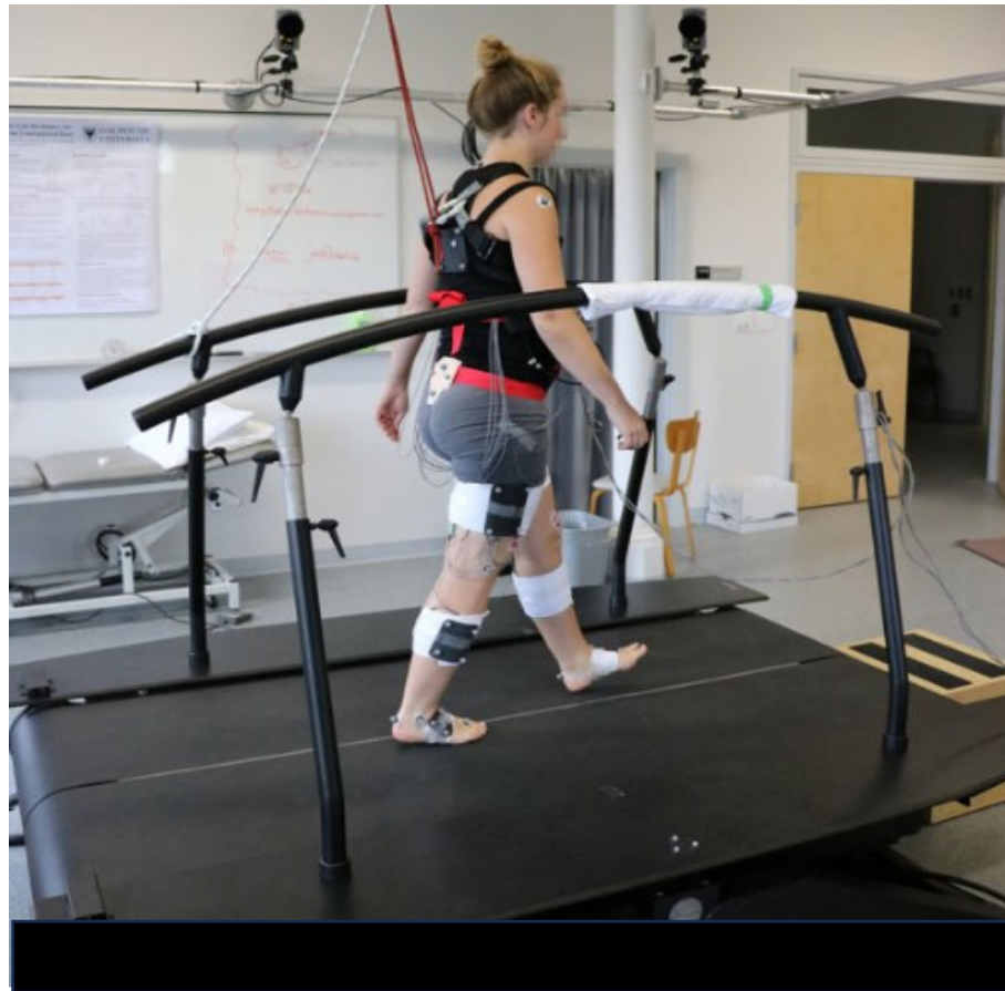
Figure 3.2: Retro-reflective marker locations during treadmill walking for key lower extremity and pelvic and spinal markers. Combat boots not pictured. (From Rutherford et al. [181] with permission Sage, 2023)
