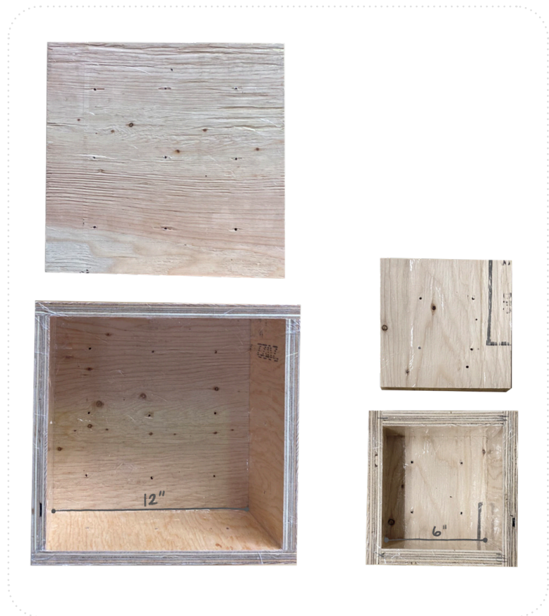
Form A (left) for 12"x12" experiments, Form B (right) for 6"x6" experiments.
