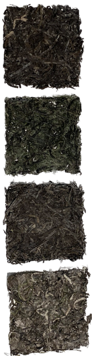
Small scale (5 g) eelgrass sheet tests done before larger sheet experiments.
