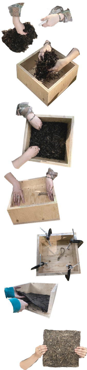
Process of compressing eelgrass sheet experiments.
