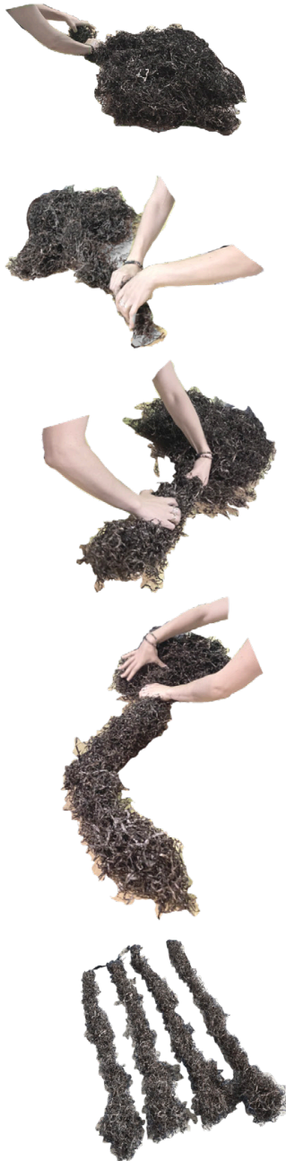
Process of twining eelgrass for thatching experiments.
