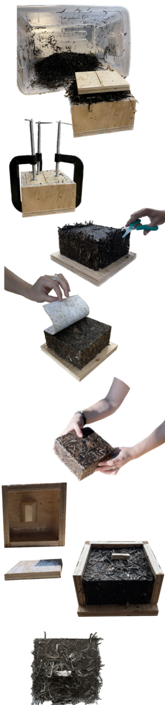
Process of compressing eelgrass block experiments.
