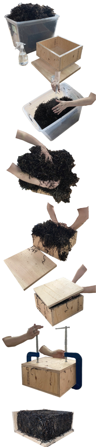
Process of compressing eelgrass insulation bale.
