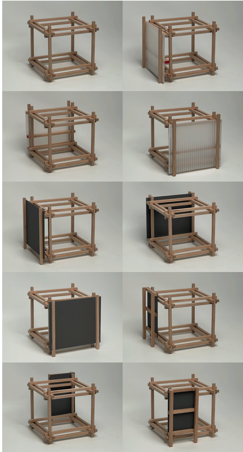
Array of 1:20 community model assembly. Building elements used to form an assembly.
