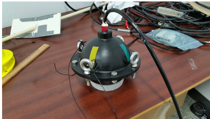
Figure 3.2: Image of the transmitter with the exterior closed. The yellow and green tapes show the coil orientations.
