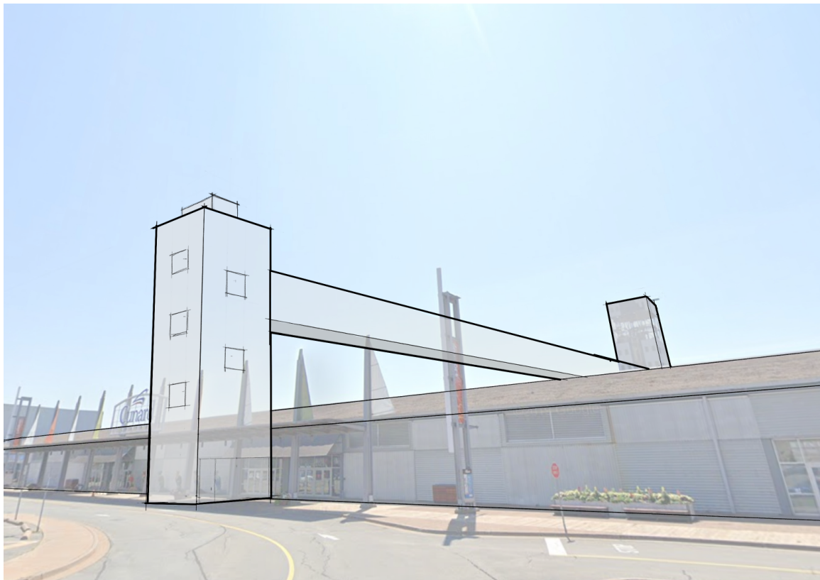
Figure 56. The support for the gantry crane doubles as another entry for the Warehouse Block. (base from Google Earth 2020)
