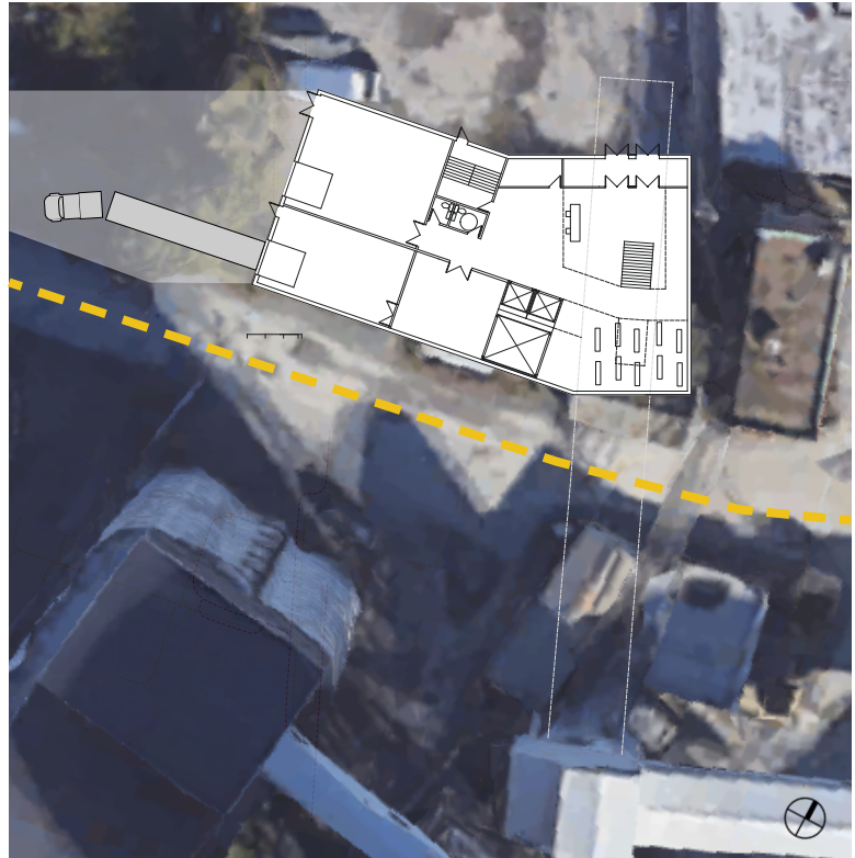
Figure 64. The Mitchell Street Artist Centre is built at the end of Mitchell Street to maintain the grain elevator's operations. To connect to the Artist Centre the conveyor is extended perpendicularly to and through the building. (base from Google Earth 2020)
