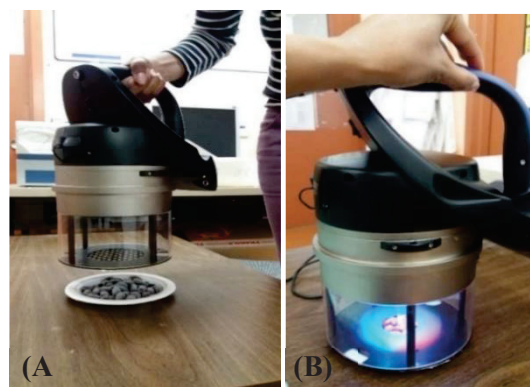
Figure 2. The Multiplex fluorescence detector. A side view of the Multiplex instrument (A), Measurement of the haskap berry skin anthocyanin in the laboratory using the Multiplex by triggering the excitation light (B)
