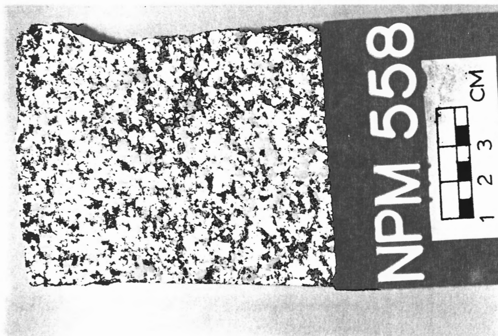
Photo 2-15: Stained hand specimen of medium-grained biotite granodiorite of Unit 4 from Port Mouton Head (interior of the pluton)
