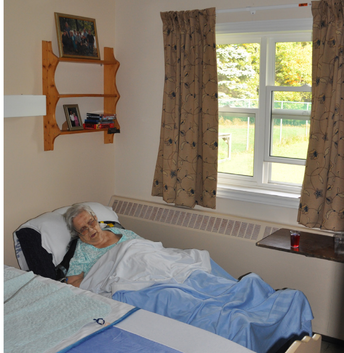
Figure 17. Lincourt Manor Nursing home, St. Stephen NB. This image shows that window heights were too high for residents to view out of from the seated position
