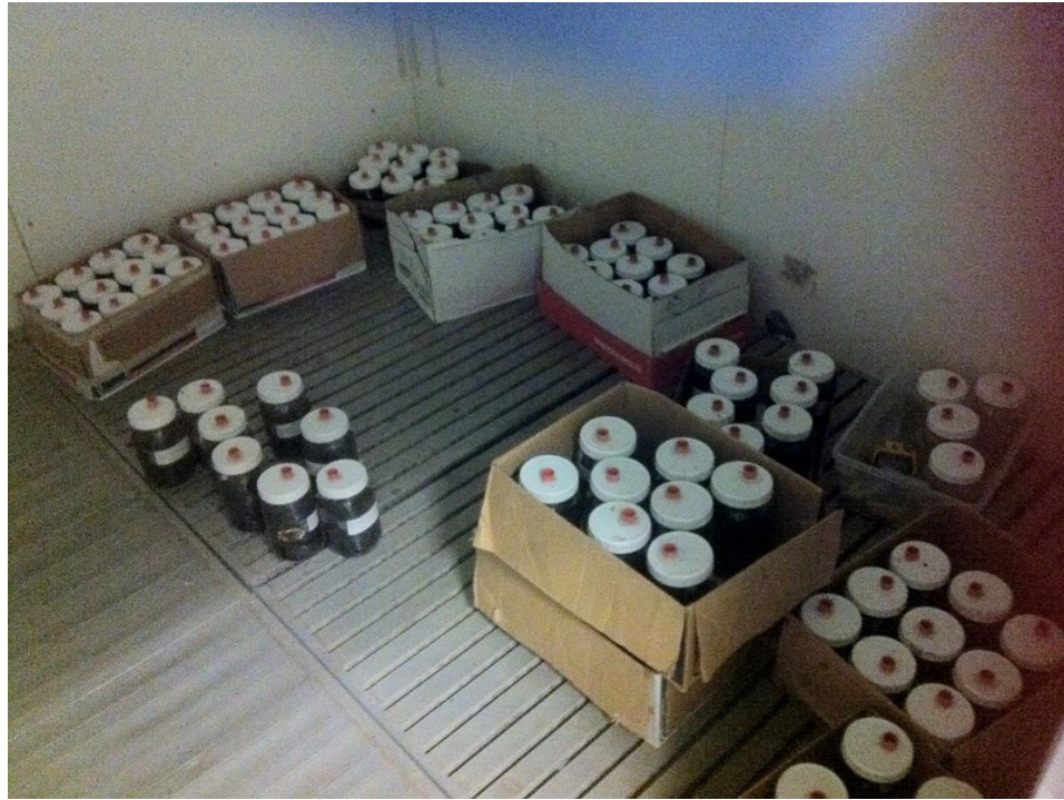
Figure 3.1 Mason jars containing compost samples inoculated and incubated at 37 °C in a walk-in incubator, Faculty of Agriculture, Dalhousie University.
