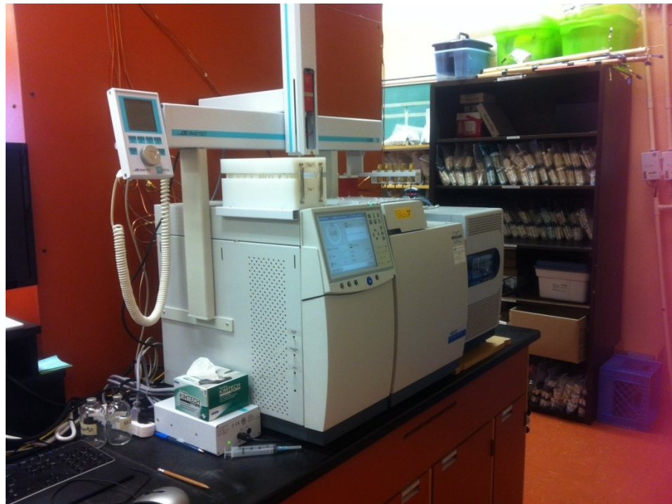
Figure 3.2 Gas chromatograph used to analyse gas samples obtained from headspace to determine CO 2 evolved from compost samples.
