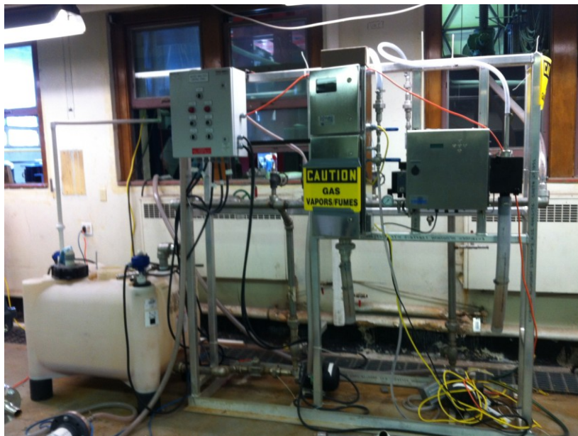
Figure 3.2: Testing loop setup showing the T200 tank (left), the Arjay monitor (center), and Sigrist monitor (right). Not shown: ASLSS and probe monitors, T100 tank.
