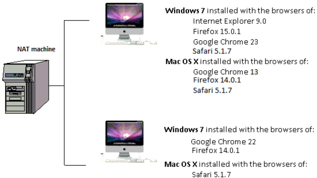
Figure 20 Two hosts are found behind the NAT device in the encrypted traffic in Nims-NAT data set
