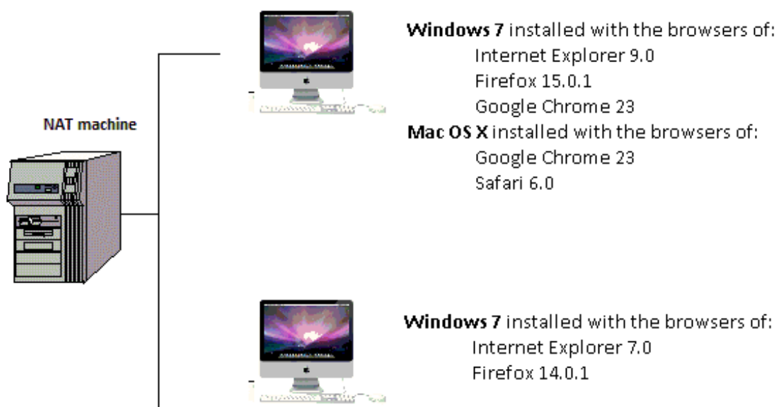
Figure 19 Two hosts are found behind the NAT device in the unencrypted traffic in Nims-NAT data set
