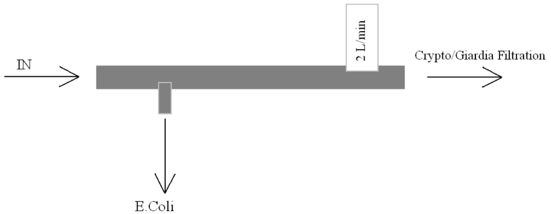
Figure 3.3 Schematic of microbial sampling apparatus
